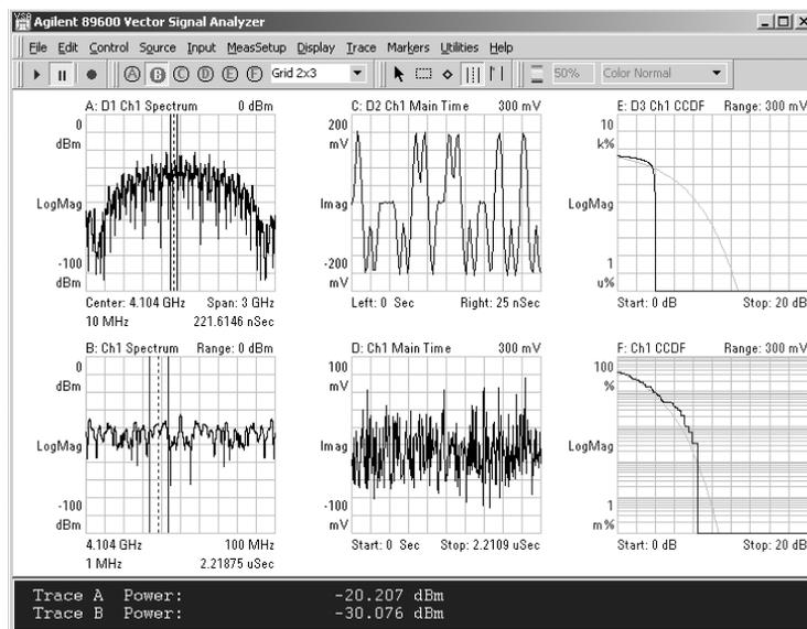
**Figure 18. Spectrum and time domain plots of a DS-UWB-like signal for 3 GHz (top traces) and 100 MHz (bottom traces) frequency spans. The lower traces of voltage (middle) and CCDF (right-hand) show the increasingly noise-like nature of the signal as the analysis bandwidth is reduced.**
