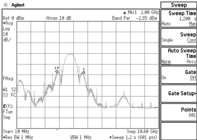
Figure 43. Mixed noise and spurious average detection.
