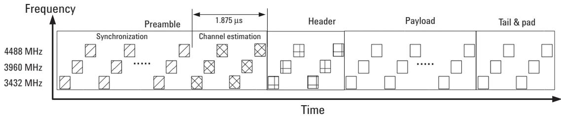
Figure 10. Frequency switching for each symbol of UWB-OFDM burst.<sup>2</sup>
