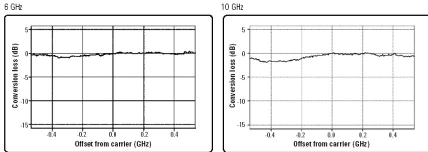
Figure 61. Specifications for PSG Option 015 wideband modulation.
