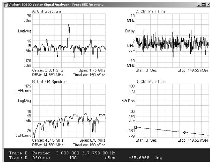
Figure 56. Using the FM demodulation in 89601.
