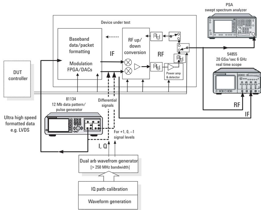
**Note:** The 2 channels of the 81134 can be used to create either 3 level pulses or I and jQ signals. Setting the dattern pattern to a long prbs (up to 2<sup>31</sup>) creates a wideband noise-like signal.
