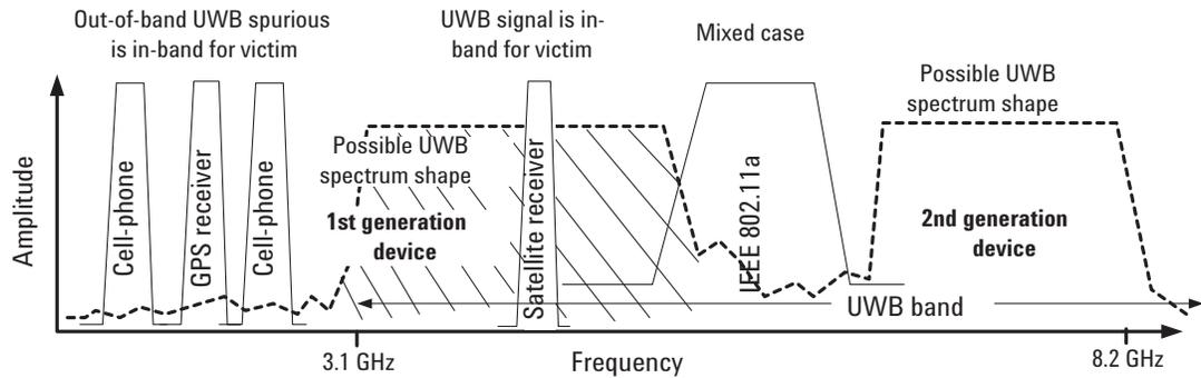
Figure 15. In-band versus out-of-band Interference for different victims.
