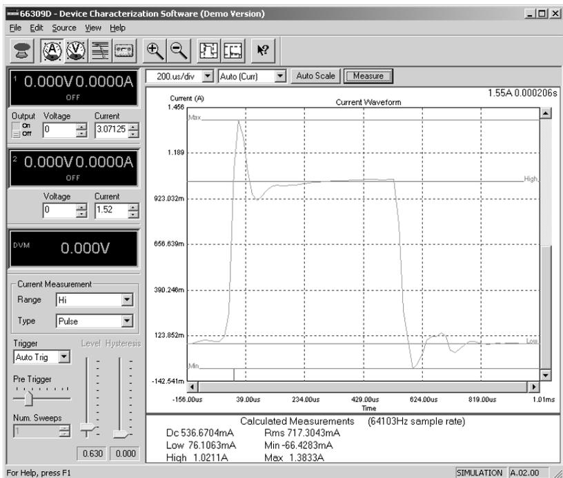
Figure 65. Sample plot of the 14565A software.
