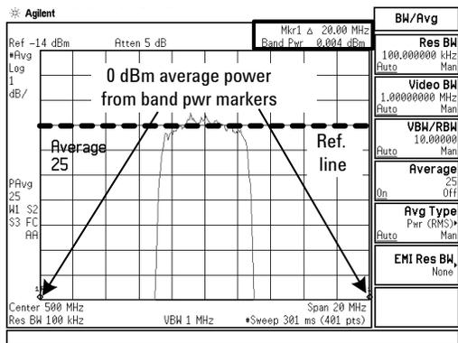
Figure 36a. A 5 MHz noise source on a 500 MHz carrier.
