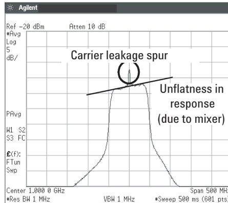
Figure 35. An example of poor PSD flatness.
