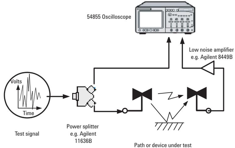
Figure 21. Using digitized signal for time correlation/coherence measurements.
