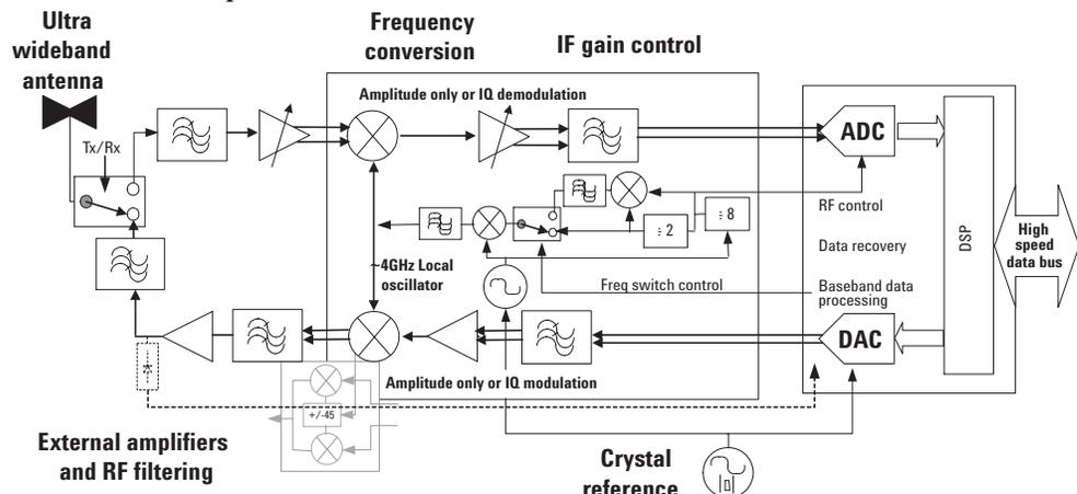
Figure 9. Block diagram of OFDM UWB radio.
