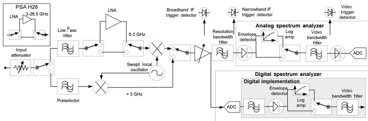
**Figure 45. Block diagram of a swept spectrum analyzer. Like any tuned receiver, the local oscillator is tuned to select specific frequencies. The output of the signal mixer is fed to either analog or digital processing. In this diagram, the switching path for frequencies above 3 GHz is also shown.**
