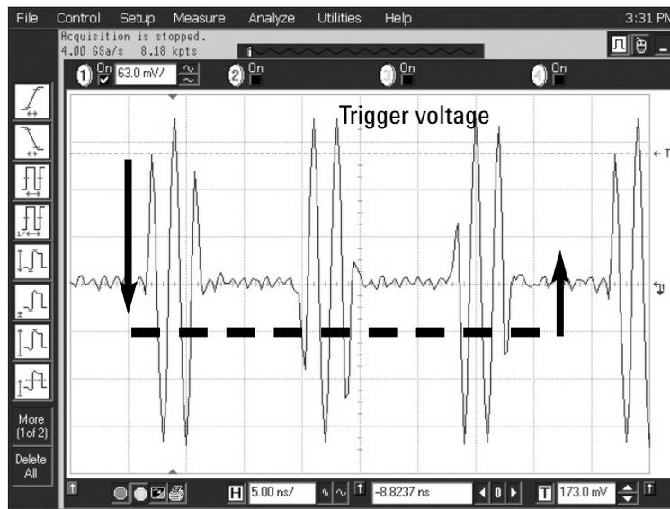
$$T_{\text{Holdoff}} = n/\text{PRF} - 1/f_{\text{RF}} \\ = 3/75 - 1/400 \mu\text{s} = 37.5 \text{ ns}$$
