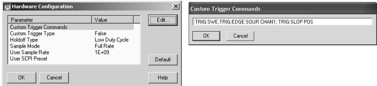
Figure 32. Entry fields for complex trigger commands in 89601.
