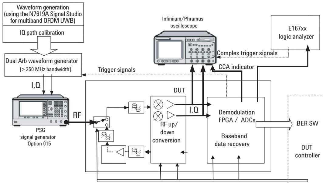
Figure 62. Enhanced receiver test configuration for EVM measurements.
