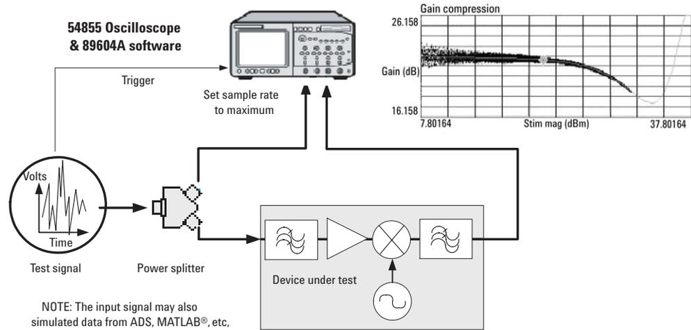
Figure 24. Test configuration for using 89604 distortion suite.
