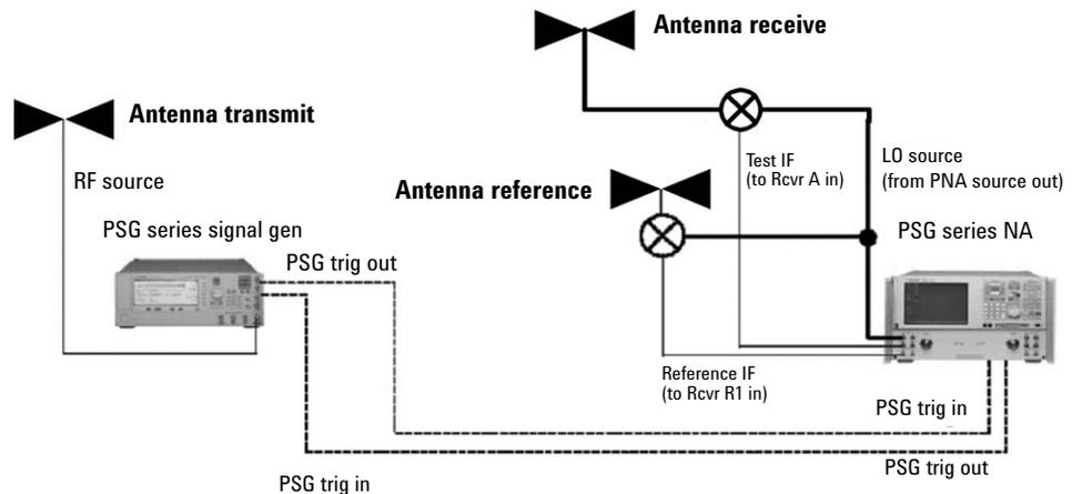
Figure 20. Extended range test configuration for antenna pattern and channel response measurements, using a vector network analyzer and triggered external RF source.
