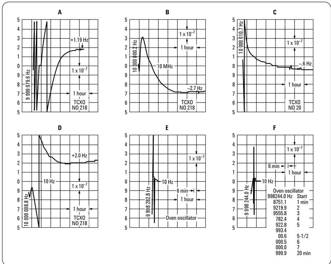
**Figure 1.** Graphs A, B, and C show how three similar crystals have very different turn-on characteristics. Graphs A and D show how the same crystal will exhibit different turn-on (retrace) characteristics. Finally, graphs E and F show the improved turn-on stability of an OCXO.
