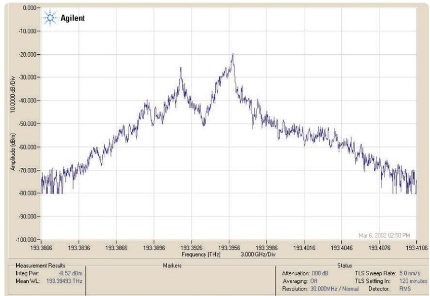
Figure 5. Agilent 83430A spectrum (using High Resolution Spectrometer)
