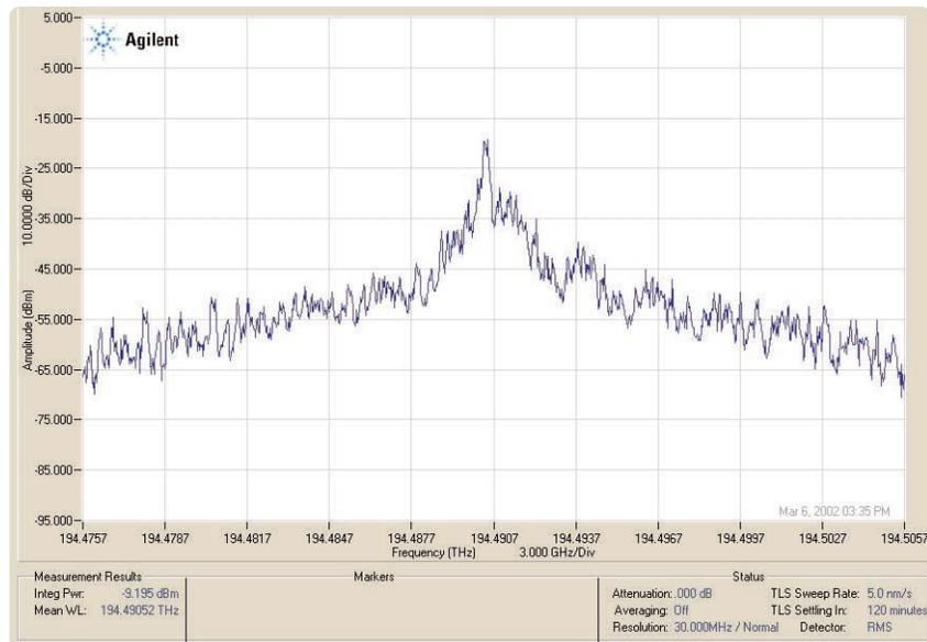
Figure 8. EML spectrum (using High Resolution Spectrometer)
