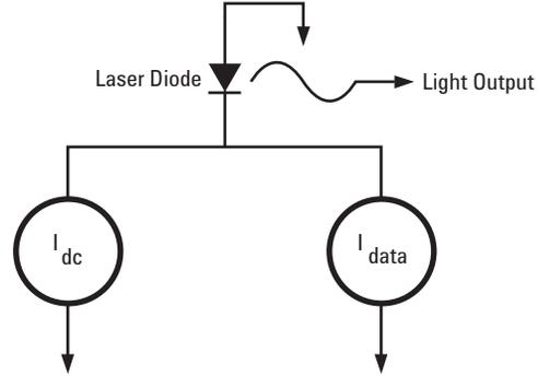
**Figure 3. Direct modulated DFB laser**
