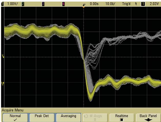
Figure 1. Infrequent metastable state captured on Agilent’s MSO6000 Series oscilloscope using real-time sampling.
