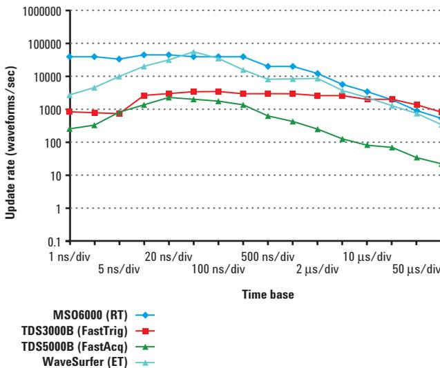
Figure 7. Each scope's fastest waveform update rate mode as a function of time base setting.
