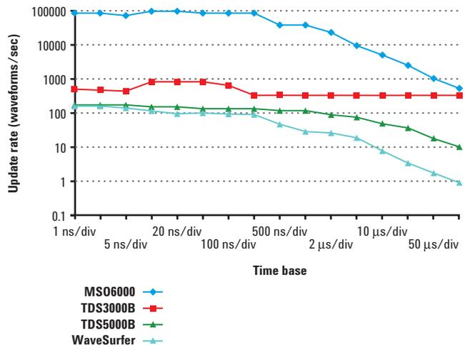
Figure 8. Waveform update rates using each scope's default real-time sampling mode.
