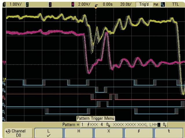
Figure 2. Pattern triggering reveals a setup-and-hold-time violation.
