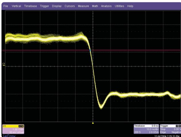
Figure 5. The LeCroy 400 Series scope fails to capture the metastable state after 10 seconds using real-time sampling.
