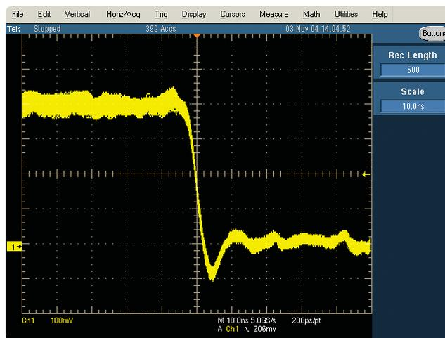
Figure 4. The Tektronix TDS5000B Series scope fails to capture the metastable state after 10 seconds using real-time sampling.
