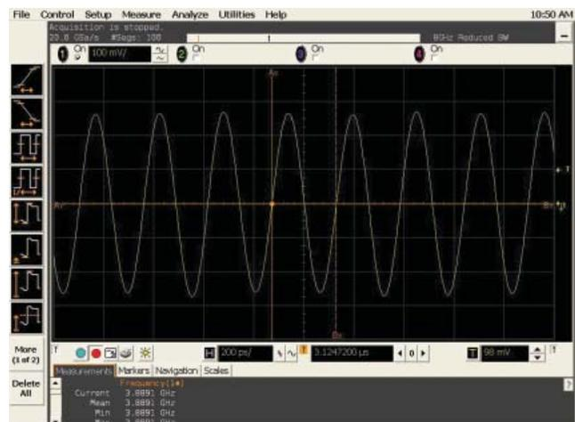
Figure 4. Expanding a segment and measuring frequency
