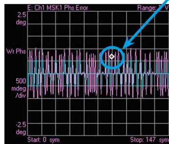
Figure 46. IQ phase error display
