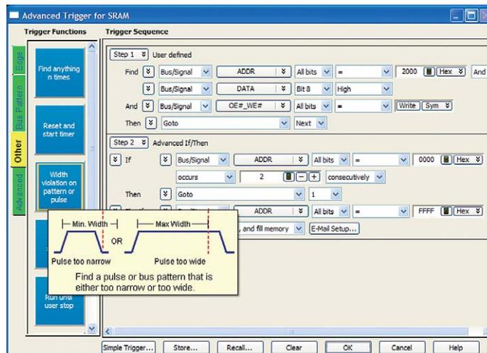
**Figure 12. Customize a trigger to specify the sequence of events leading up to a trigger event.**
