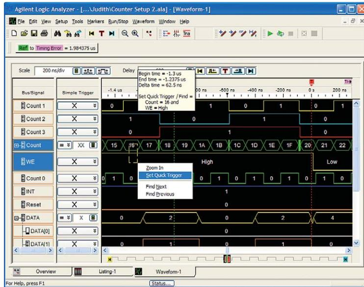
Figure 11. Create a trigger by simply drawing a box around an event in the current trace.
