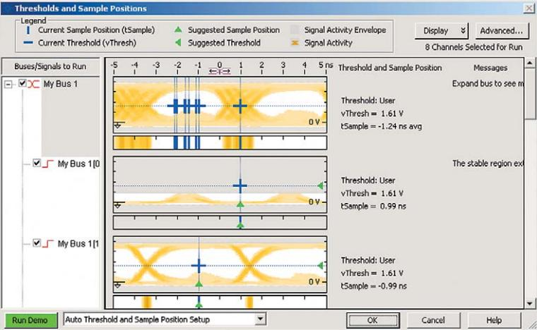
Figure 5. Identify problem signals quickly by viewing eye diagrams across all buses and signals simultaneously.
