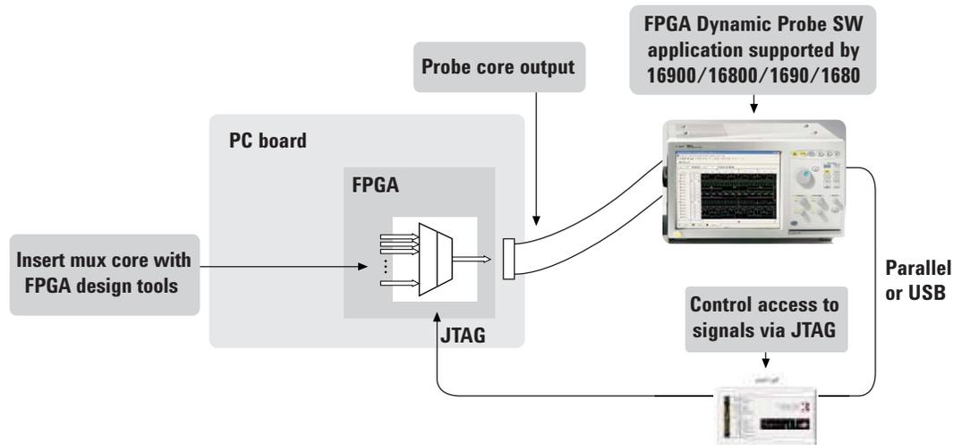
Figure 2. Create a timesaving FPGA measurement system. Insert an ATC2 (Agilent Trace Core) core into your FPGA design. With the application running on your logic analyzer you can control which group of internal signals to measure via JTAG.
