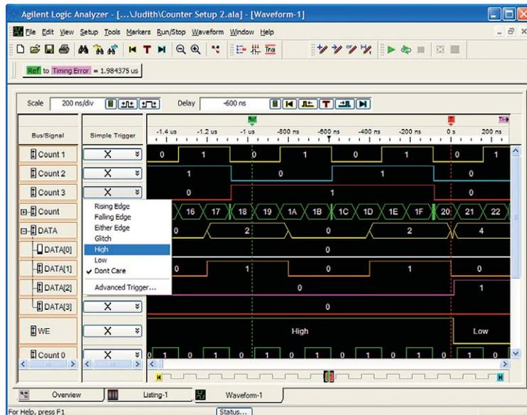
**Figure 10.** Define a single trigger event as a combination of levels, edges, patterns or glitches across multiple signals and buses.
