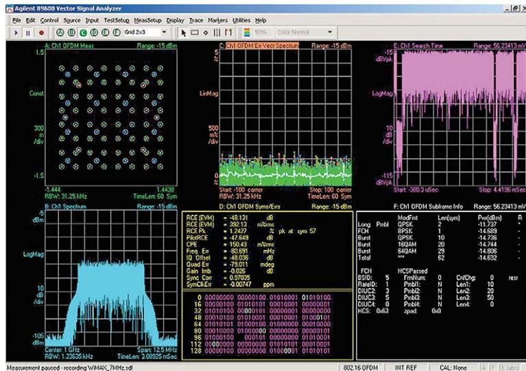
Figure 7. Perform in-depth time, frequency, and modulation domain analysis on your digital baseband and IF signals. Agilent's 89600 vector signal analysis software provides flexible tools for making quality RF and modulation measurements on digital communication signals.
