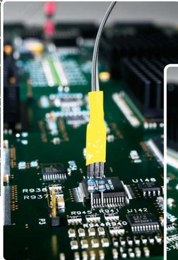
...probe a pin of a QFP package
