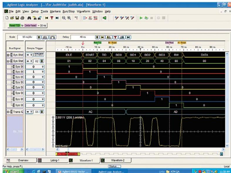
Figure 6. View Scope integrates time-correlated oscilloscope and logic analyzer waveforms into a single waveform display.
