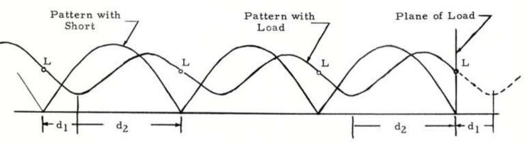
Input Impedance = Load Impedance at Points Marked "L".
