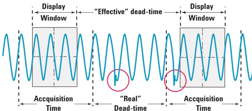
Figure 1. Oscilloscope dead-time versus display acquisition time.
