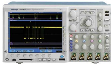
**Figure 8. Tek's MSO4104 fails to capture and decode CAN error frames with a software-based decoding update rate of just one 1 decode every 5 seconds.**
