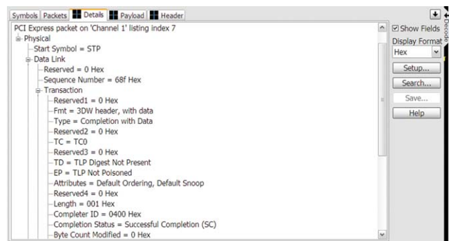
Figure 6. A Details Tab clearly shows the Physical, Data Link and Transaction Layers of a high speed protocol
