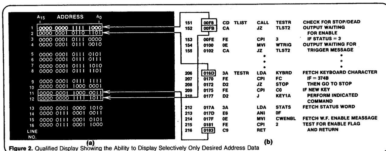
displays the address of the CALL instruction, 00FB. Therefore, during the next four machine cycles: the high-order 8 bits of the next instruction address are stored in the push-down stack; the low-order 8 bits of the next instruction address are stored in the push-down stack; the stack pointer is decremented by 2; and control is transferred to the first address of the subroutine.
