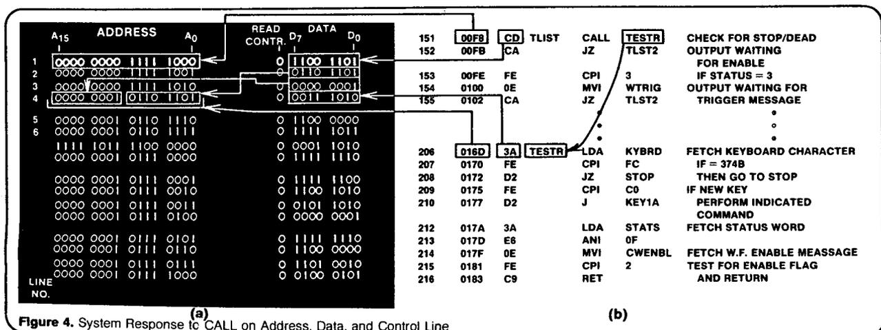
Figure 4. System Response to CALL on Address, Data, and Control Line
