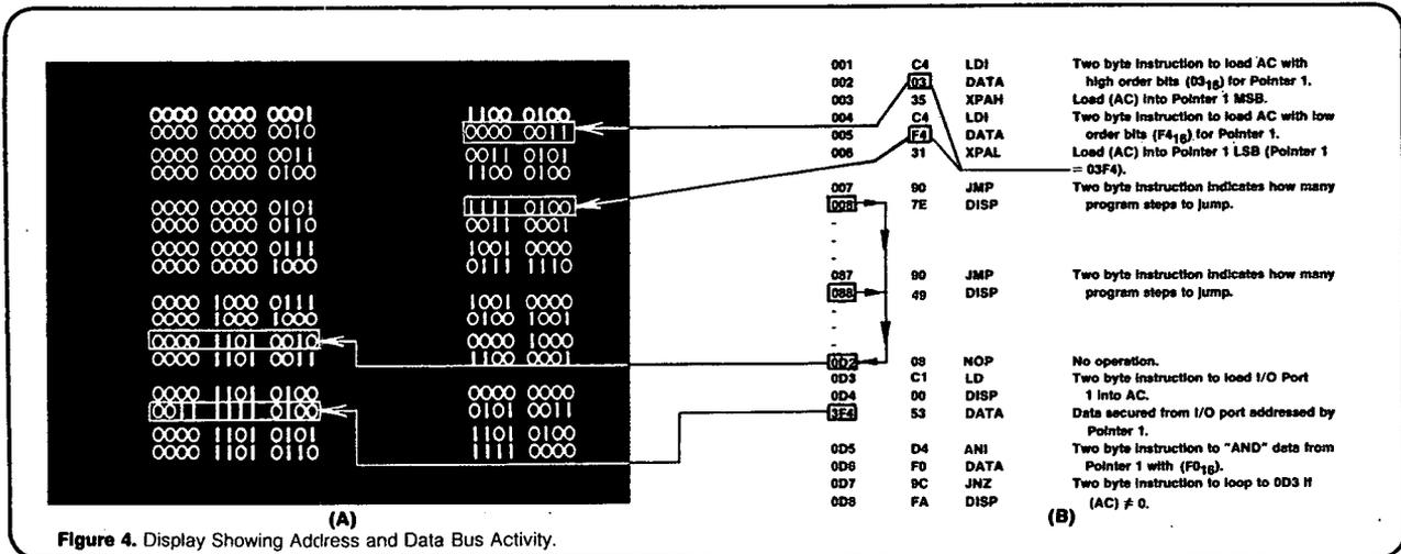
Figure 4. Display Showing Address and Data Bus Activity.
