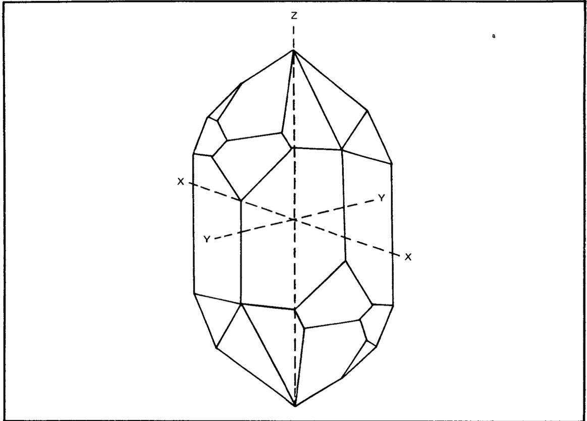
Figure 4. Doubly terminated quartz crystal showing axis orientation.
