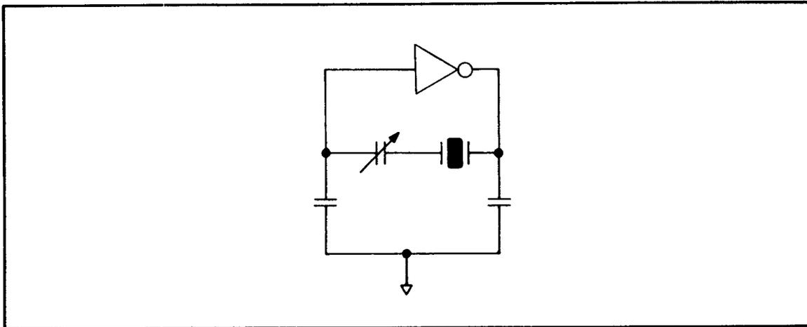
*Figure 11. The Series Resonant Oscillator*
