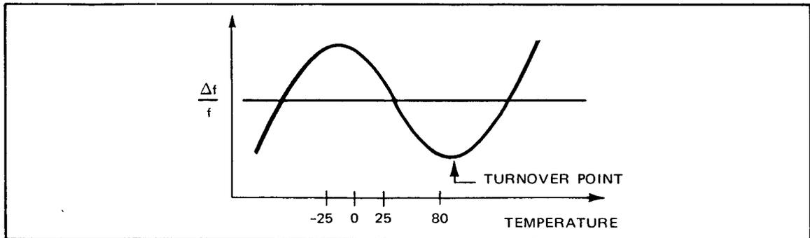
*Figure 24. Selection of oven turn over point based upon the crystal characteristic curve.*
