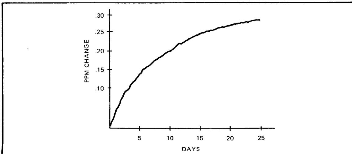
Figure 15. Time domain stability of the fractional frequency change over time (days) starting from a point of calibration.
