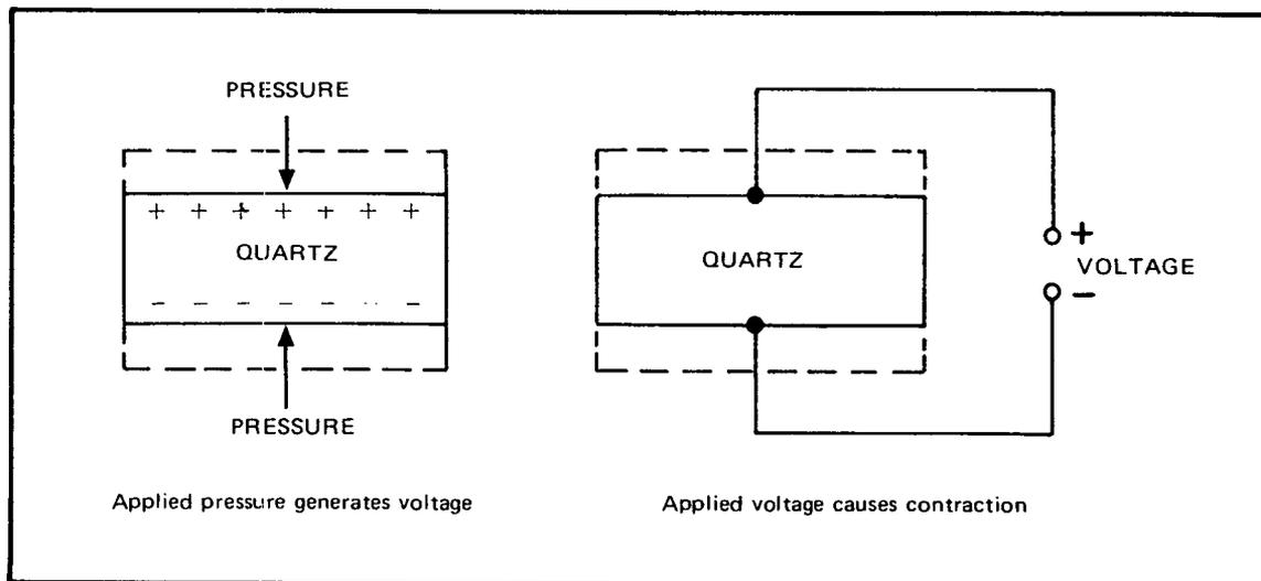
*Figure 3. Piezoelectricity principles.*
