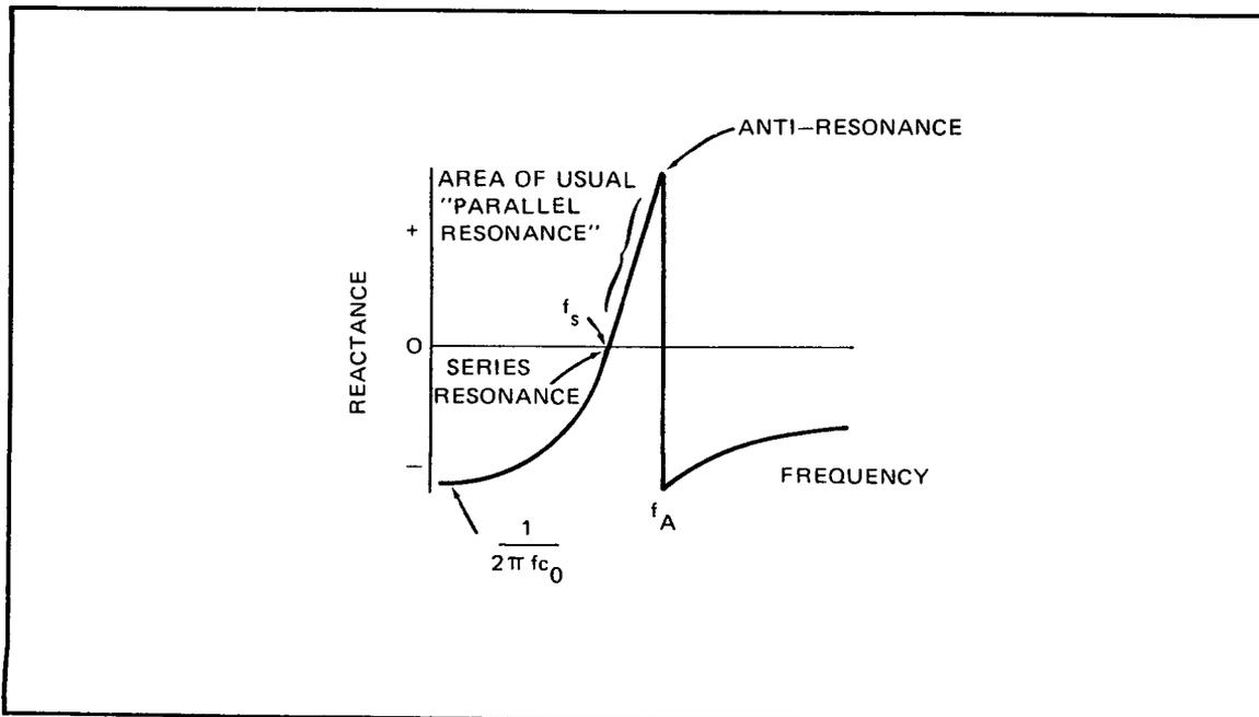
Figure 10. The reactance of the crystal varies with the frequency of operation near resonance.
