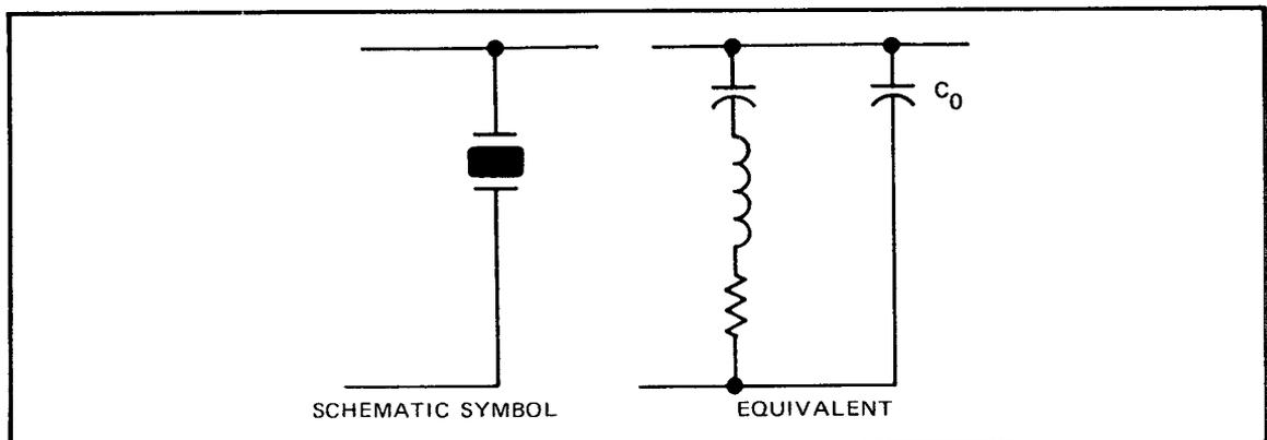
Figure 1. Equivalent circuit of a crystal includes the capacitances contributed by the wire leads and the holder in  $C_0$ .
