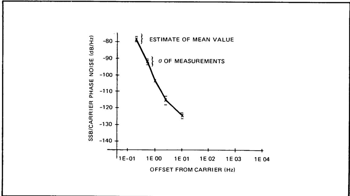
Figure 18. Phase spectral density at specific offsets from the carrier.
