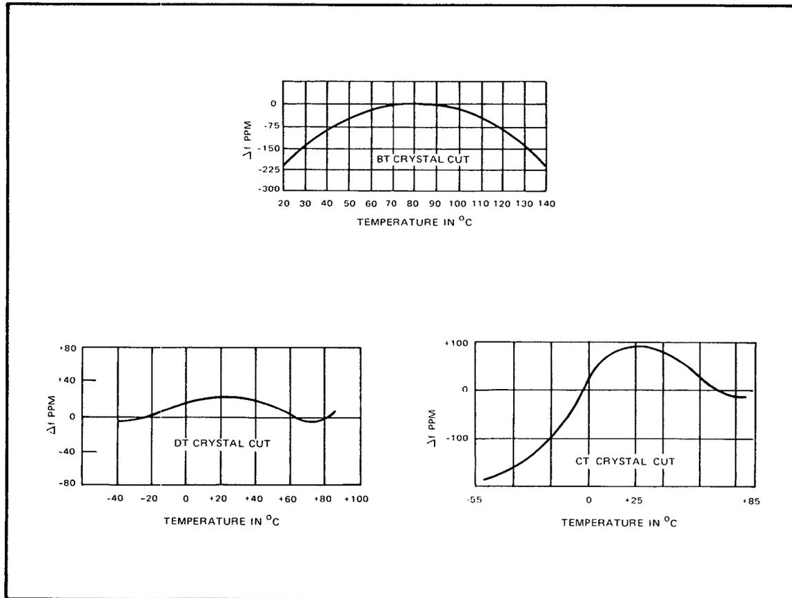
Figure 13. Frequency vs. temperature plots for DT, BT, and CT cuts.
