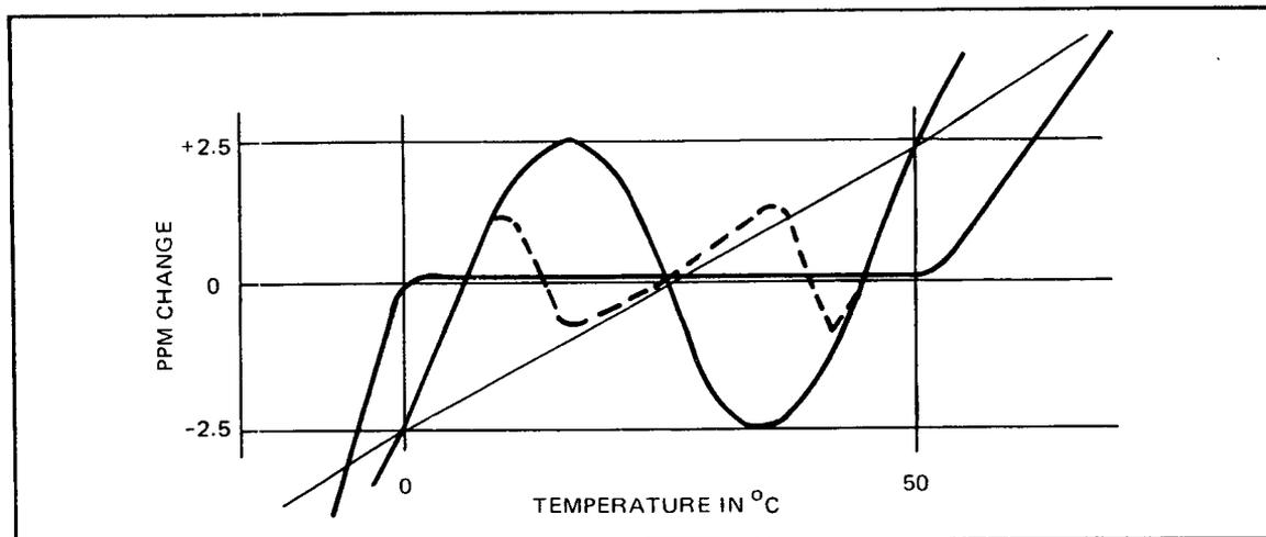
Figure 21. Frequency temperature plots for several room temperature oscillators.
