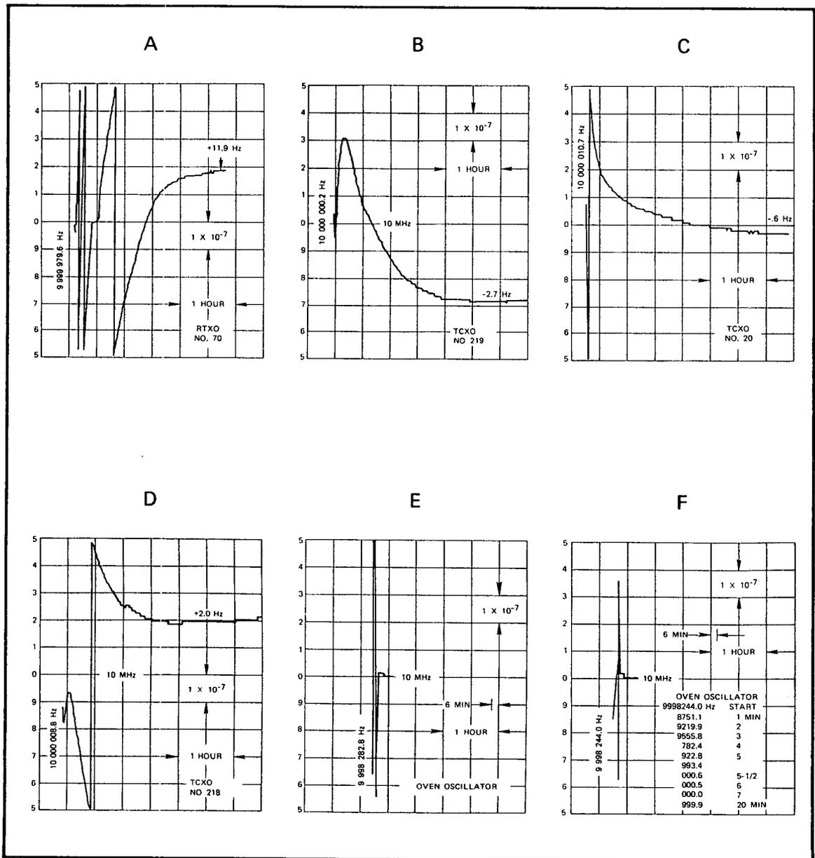
Figure 25. A is a RTXO warm up curve. B, C and D are typical TCXO warm up characteristics. The long time (3 hours) is due to changes in temperature inside the instrument. E and F are oven oscillators. Stability is achieved in  $\approx 20$  minutes.
