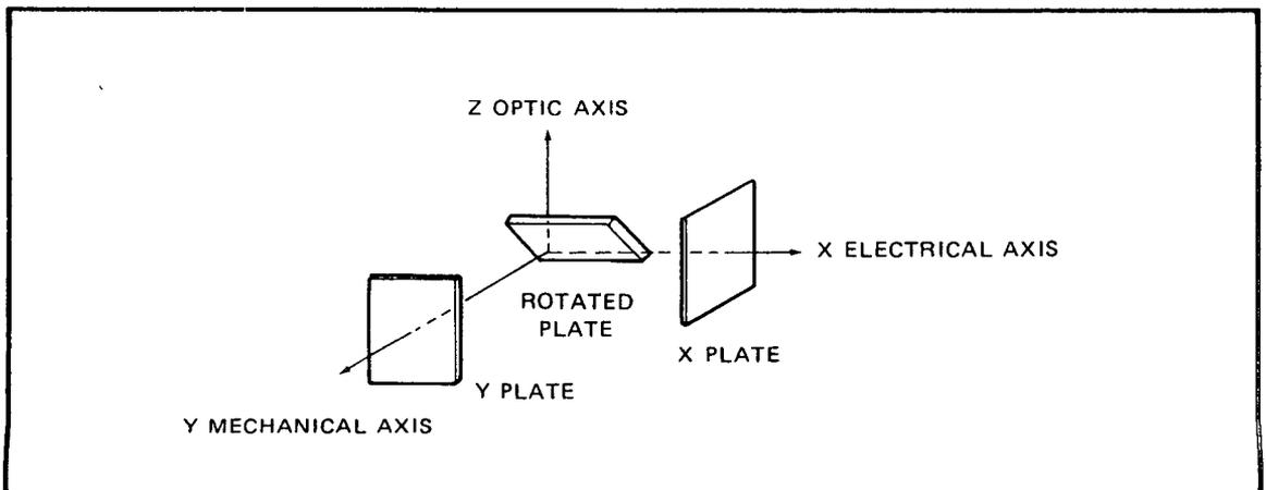
Figure 5. A description of the axis of quartz and X, Y, and rotated plates.
