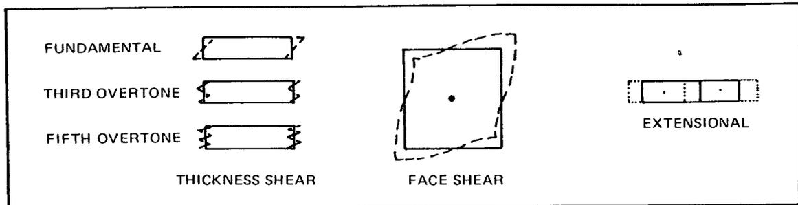
Figure 7. Vibration modes of various crystal cuts and the thickness shear overtone.
