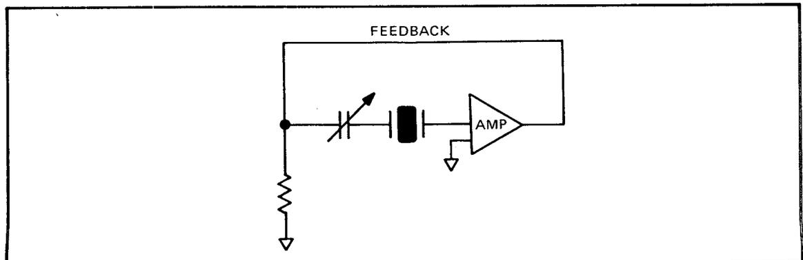
Figure 2. Simplified amplifier feedback (oscillator) circuit using a crystal resonator.
