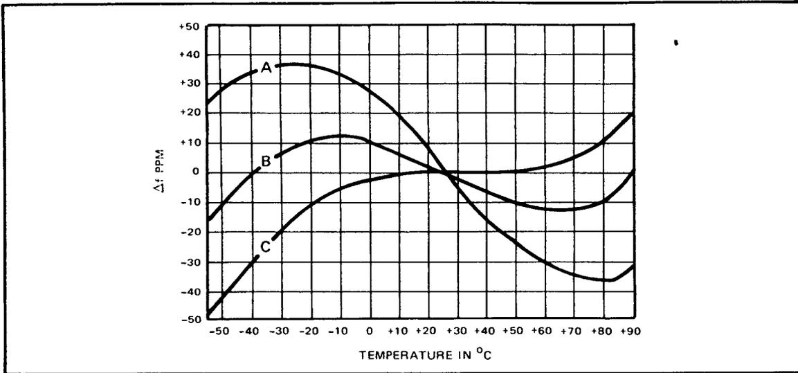
Figure 14. A, B, and C are temperature vs. frequency plots of AT cuts which have been varied by a few seconds of angle rotation.
