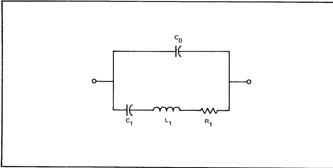
Figure 9. The electrical equivalent circuit for a crystal resonator.
