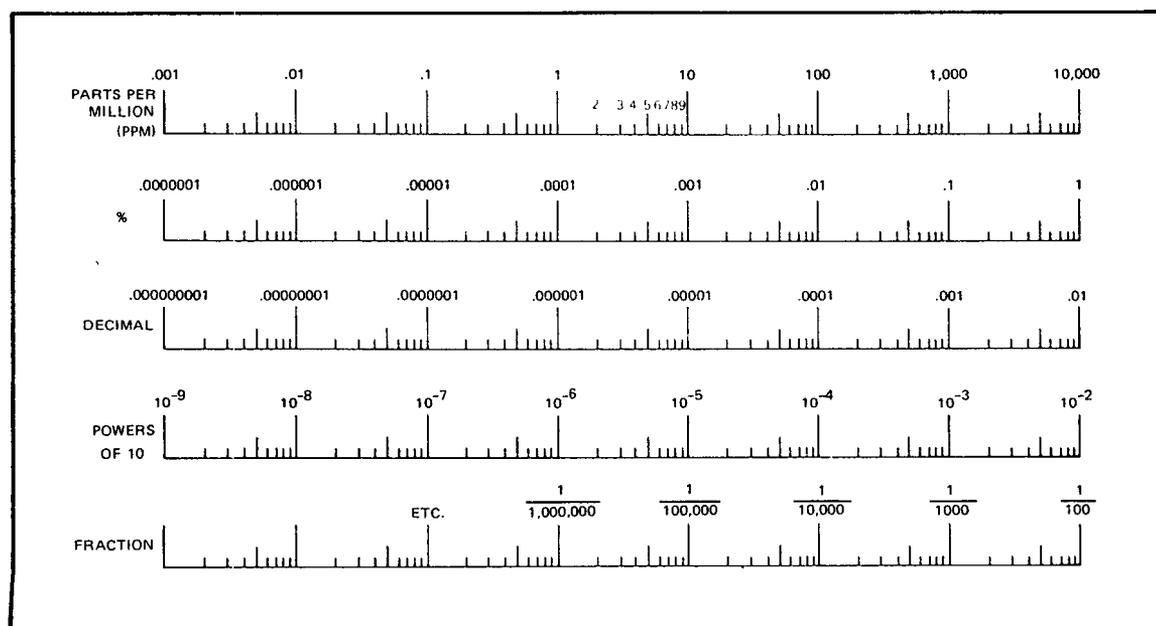
Figure 20. These factors are specified in various ways: parts per million (PPM), percent, as a deviation from a nominal frequency expressed as some power of 10, or as a fraction.
