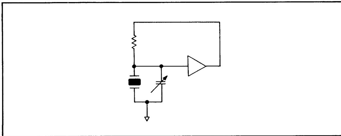
*Figure 12. The Parallel Resonant Circuit*
