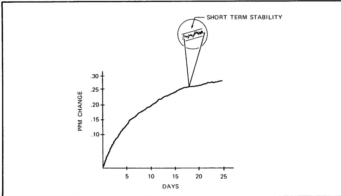
Figure 16. Short-term time domain stability or the fractional frequency change over time (seconds) and its relationship to aging.
