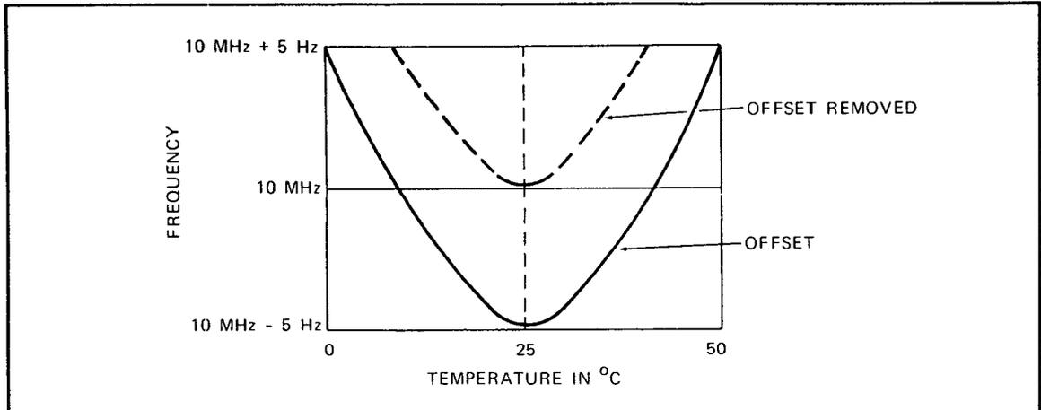
*Figure 23. The adjustment of this TCXO for compliance with temperature over its full range results in a frequency offset at 25°.*
