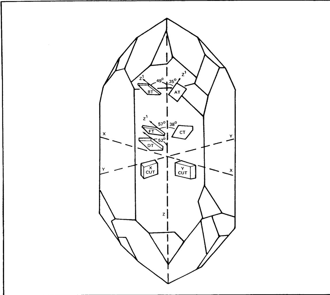
Figure 6. Typical crystal cuts from a doubly terminated quartz crystal.
