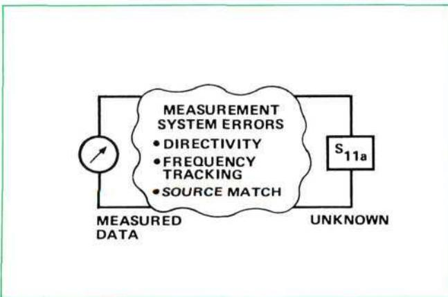
Let's consider measurement of some unknown's reflection coefficient (or return loss). No matter how careful we are, the measured data will differ from the actual. These are the major sources of error.
