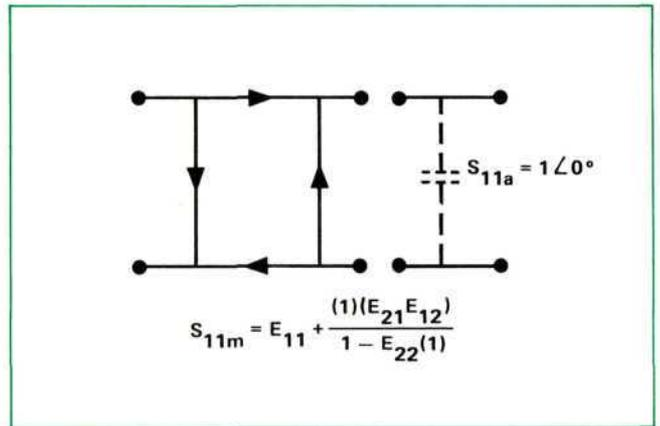
The OPEN gives us the second condition. The program can compensate for the residual fringing capacitance at the open connector.
