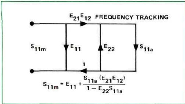
FREQUENCY TRACKING error,  $E_{21}E_{12}$ , is caused by small variations in gain and phase flatness vs. frequency (frequency response error) between the test and reference channel signals due to imperfectly matched cables, differences between incident and test couplers and in the converter, etc. It can be shown that these three errors are mathematically related to the actual ( $S_{11a}$ ) and measured data ( $S_{11m}$ ).
