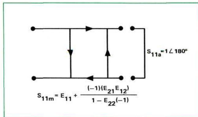
Then a SHORT circuit termination is used for the first condition of a two equation, two unknown solutions to determine  $E_{22}$  and  $E_{21}E_{12}$ .
