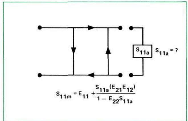
We now MEASURE the unknown  $S_{11a}$  and store the measured data  $S_{11m}$  at each frequency.
