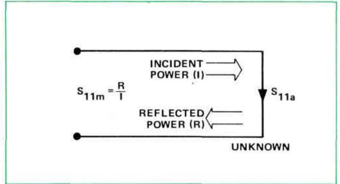
REFLECTION COEFFICIENTS are measured by first separating the incident power (I) from the reflected power (R) and then taking the ratio of the two values.
