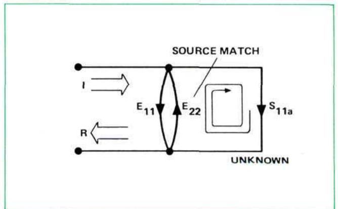
Since the measurement system test port is never exactly the characteristic impedance (normally 50 ohms), some of the reflected signal bounces off the test port and back to the unknown, adding to the original incident signal (I). This re-reflection effect is called SOURCE MATCH error,  $E_{22}$ .
