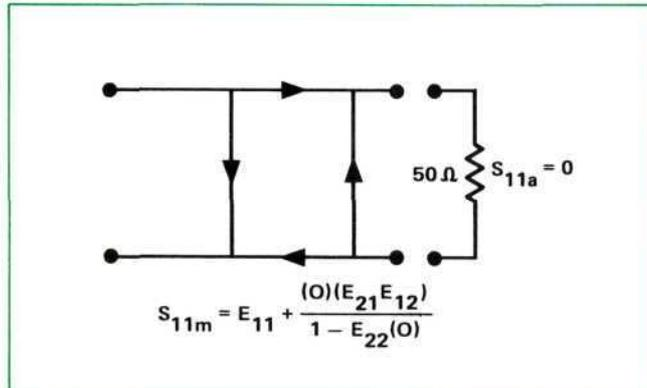
If we knew the three "E" errors at each frequency we could remove them mathematically from our measured data. They are found by measuring (calibrating) with three independent standards whose  $S_{11a}$  is known at all frequencies.
