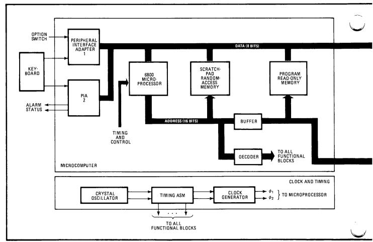
2. Shared facilities. In the 1377, the microprocessor, display refresh ASM, and the communications ASM share buses and the display memory. A major challenge is finding a way to independently analyze how these blocks work through the shared facilities.
