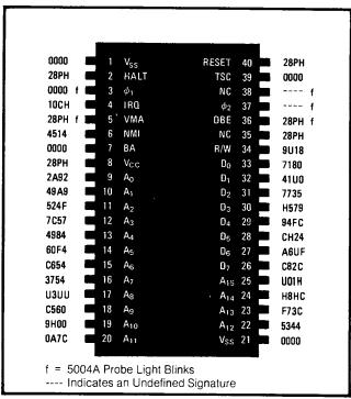
**3. 6800 pin signatures.** Running the 5001's test 00 on a good 6800 yields the above set of signatures. A good signature at pin 2 is enough to indicate that the processor kernel is operational; other signatures can be taken if further testing indicates a problem.
