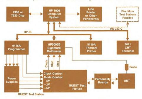
Fig. 1. GUEST is interfaced to the controlling HP 1000 via the HP-IB (IEEE 488), and to the unit under test by a personality board.
