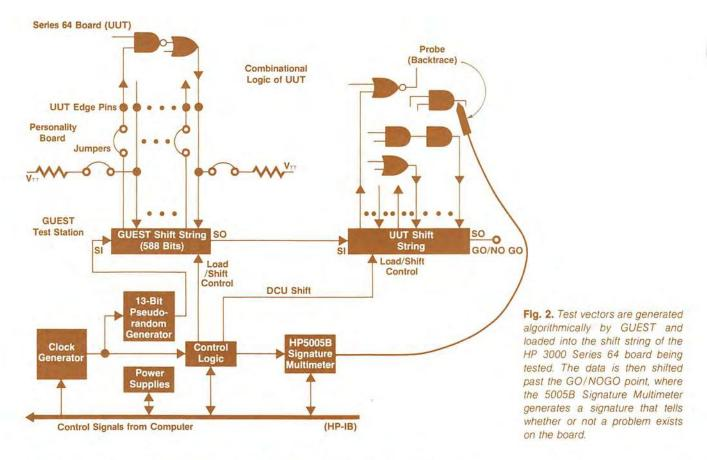
pseudorandom sequence and each output of every shift string flip-flop on the board is also driven by all 8191 bits.
