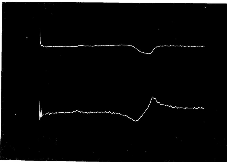
FIG 9.  $H_C$  FOR IMPACT TEST SYSTEM — Compensation curve calculated from calibration mass system.
