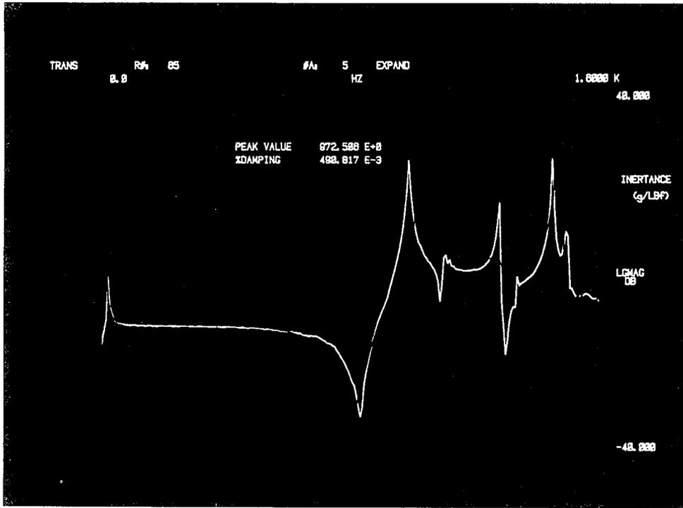
**FIG 10. EFFECTS OF ACCELEROMETER LOADING — Accelerometer too massive —** Black trace shows transfer function measurement with one accelerometer, White trace shows same measurement with accelerometer mass doubled. Comparison shows that this accelerometer was too massive for the disk brake structure under test.
