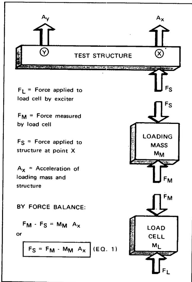
FIG 3. FORCES ACTING ON THE TEST SYSTEM — Equation 1 shows that the force actually applied to the structure is less than the force measured due to loading.
