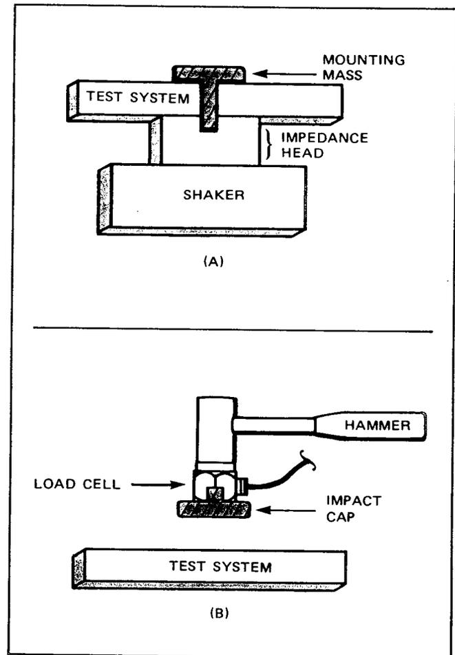
FIG 4. "REAL" MEASUREMENT SET-UPS — (A) Shaker test system, loading caused by mounting screw. (B) Impact test system, loading caused by impact cap and hardware. Force sensed by load cell differs from force applied to structure due to additional mass.
