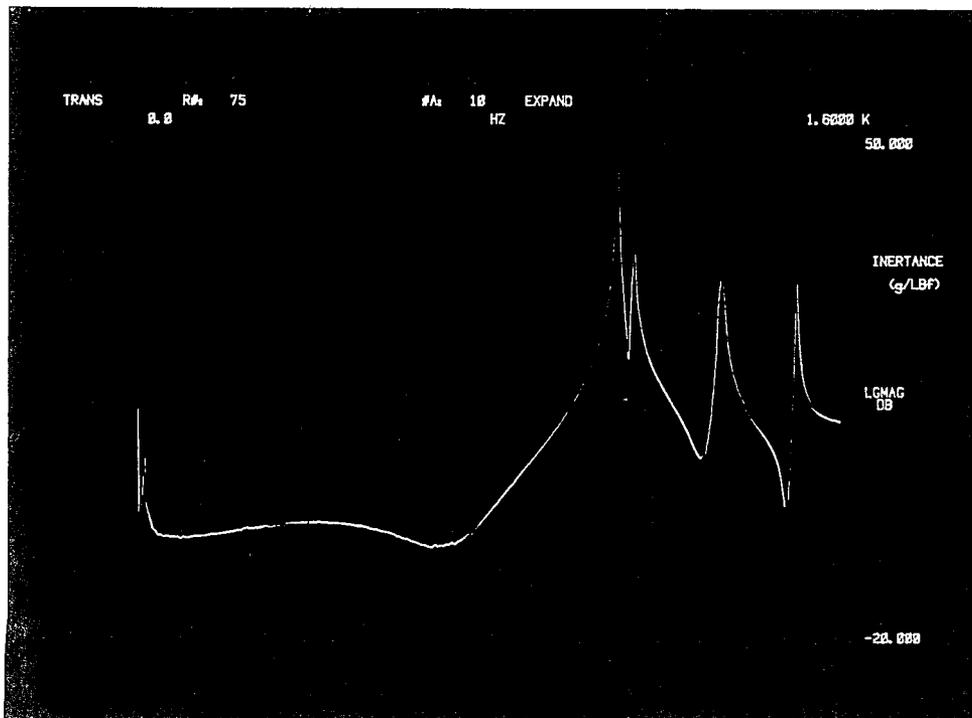
**FIG 11. EFFECTS OF ACCELEROMETER LOADING — Accelerometer OK —** Same measurements as in Figure 10, but using a smaller accelerometer. In this case, accelerometer loading is insignificant.
