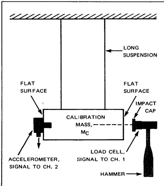
**FIG 8. CALIBRATION MASS SYSTEM** — The mass,  $M_C$ , should be large with respect to the accelerometer used. To determine the calibration curve, the mass is impacted along its center of gravity.
