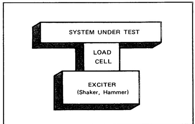
FIG 2. "IDEAL" MEASUREMENT SET-UP — Test system and exciter appear on separate sides of the load cell. Force sensed by load cell is the force actually applied to the structure.
