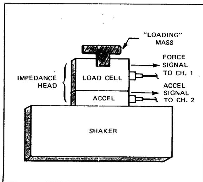
FIG 5. Test set-up used to measure effective mass of impedance head with loading mass. Resulting frequency response is  $H_I$ .
