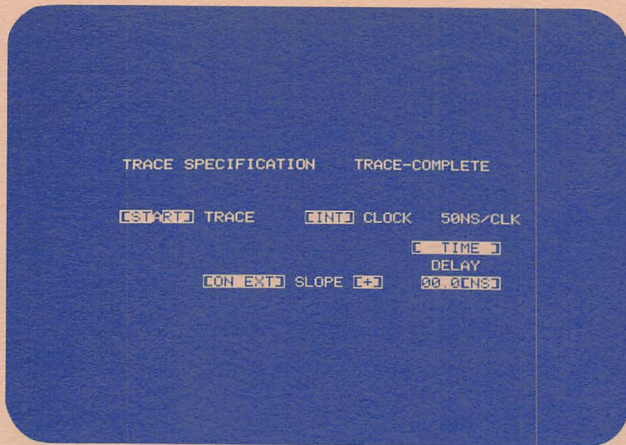
Figure 11. The [ON] field can be switched to an External trigger field which allows using the edge sensitive external trigger input on the clock pod as the trigger specification.
