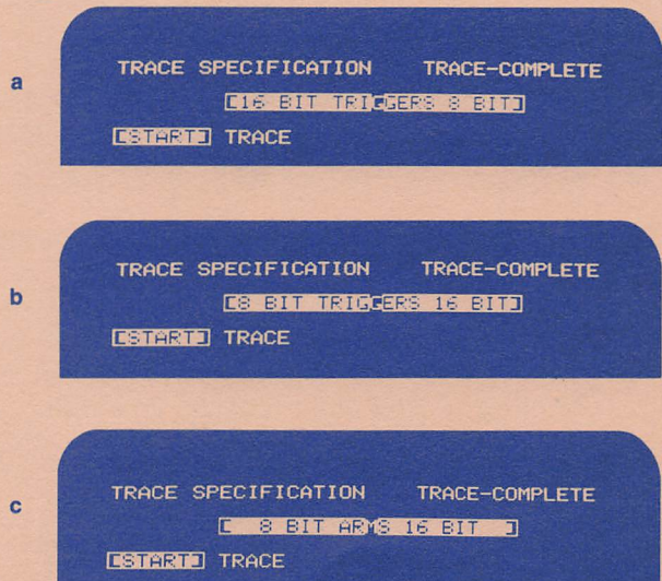
Figure 24. The analyzer may also be configured so that, upon trigger recognition, the 16 Bit machine Triggers the 8 Bit machine (a); the 8 Bit machine Triggers the 16 Bit machine (b); and the 8 Bit machine Arms the 16 Bit machine (c).
