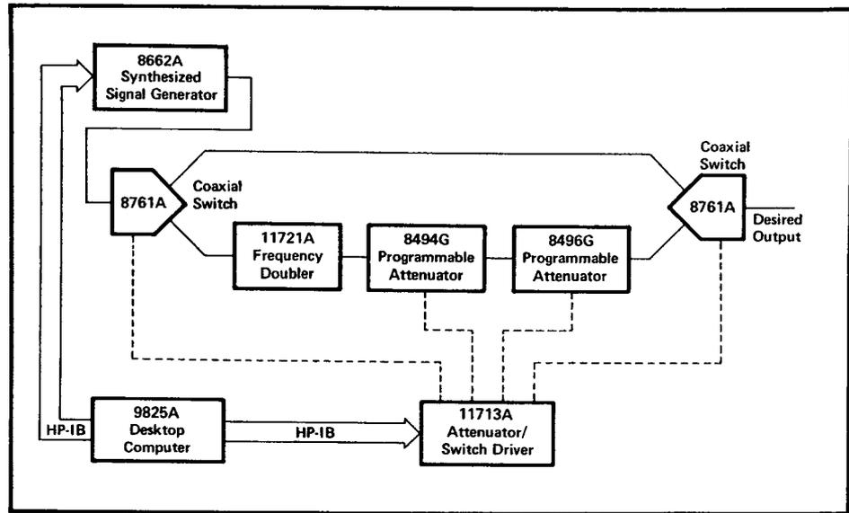
Figure 7. HP-IB System for convenient doubling control.
