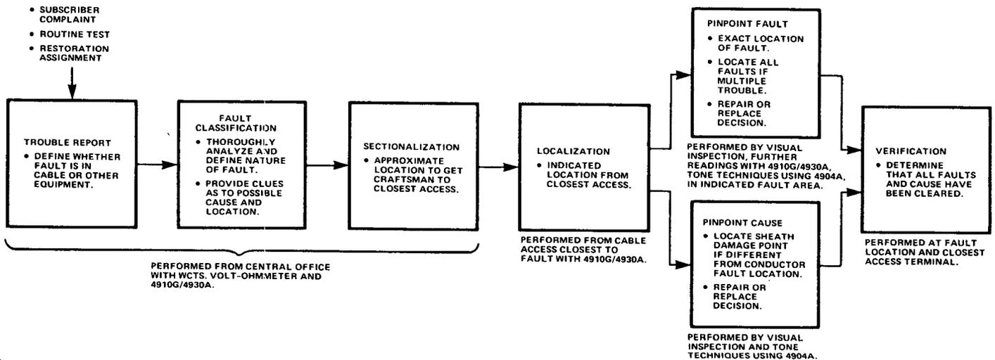
Figure 1. Fault Isolation and Repair Flowchart
