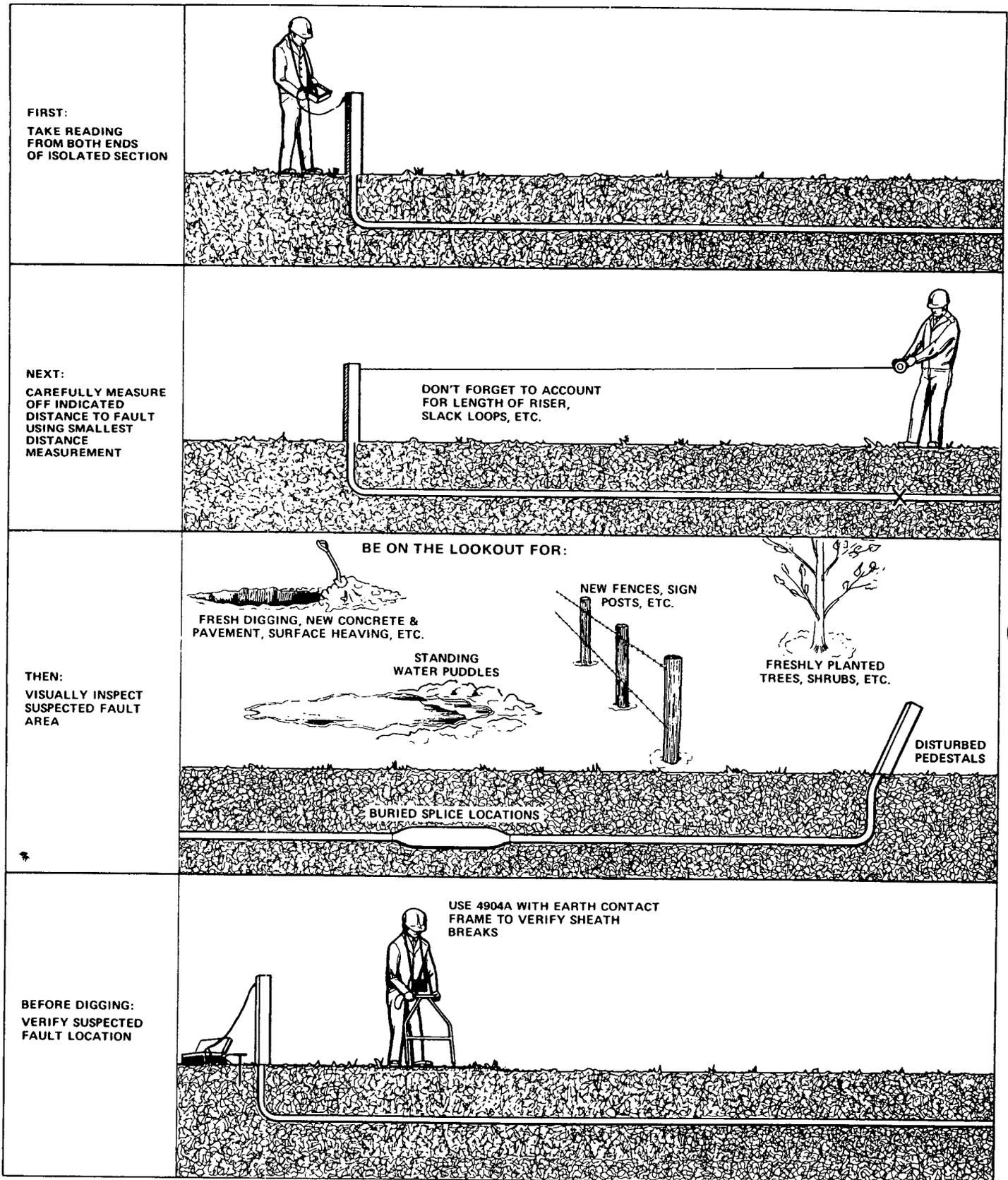
Figure 4. Pinpointing Fault Location
