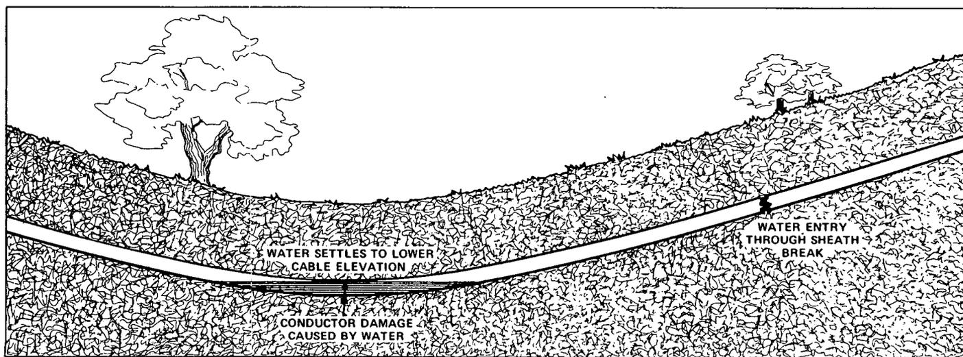
Figure 3. Water Flow in Cable
