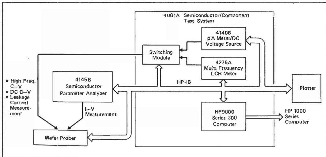
Figure 36. Automatic measurement system for CAD system
