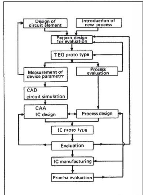
Figure 10. Flow of IC design/manufacturing
