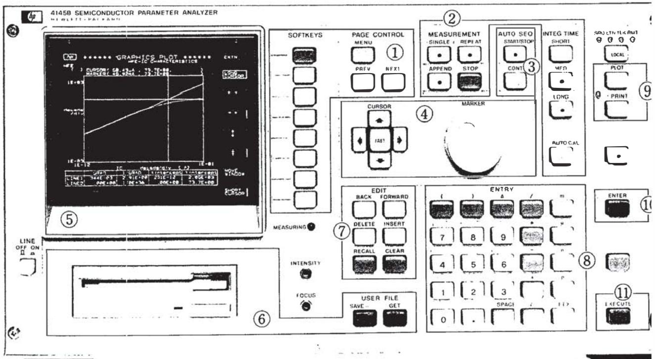
and vertical zoom-in/zoom-out ( , , , ) and for recentering ( ) the plot area. When is pressed, the plot area is automatically centered on the cursor, without changing the relative position of the cursor and plotted curves. Displayed plots can be temporarily stored and redisplayed by the and softkeys. Thus, overlay plots can be easily obtained.
