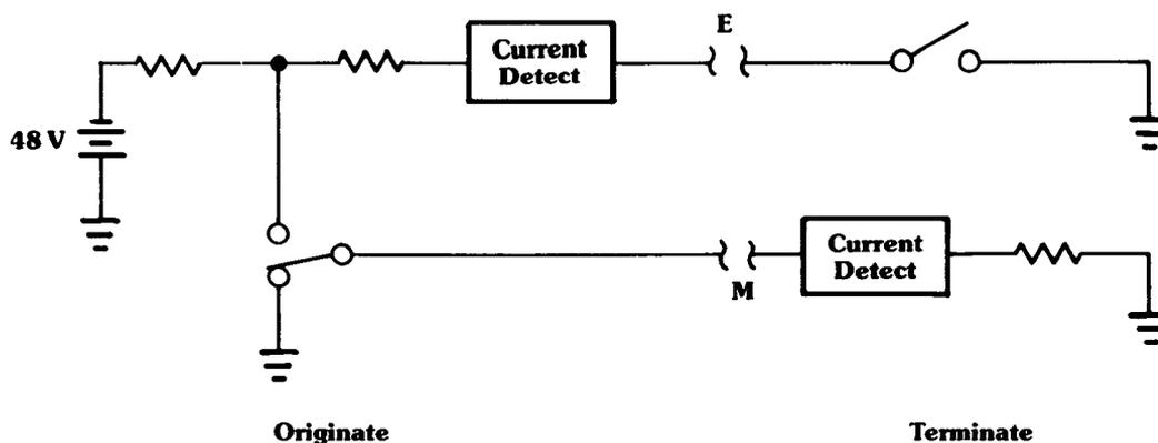
Figure 15. E/M type I signaling.
