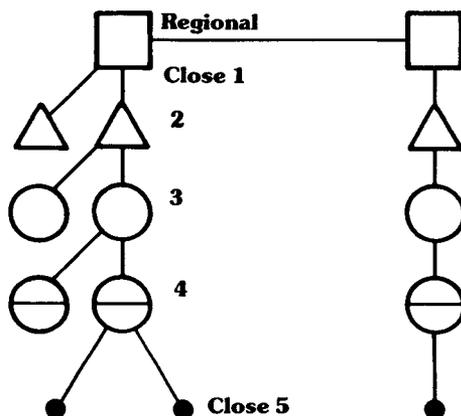
Figure 7. Five level switching system.
