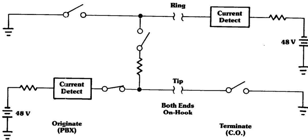
Figure 10. Ground start signaling.
