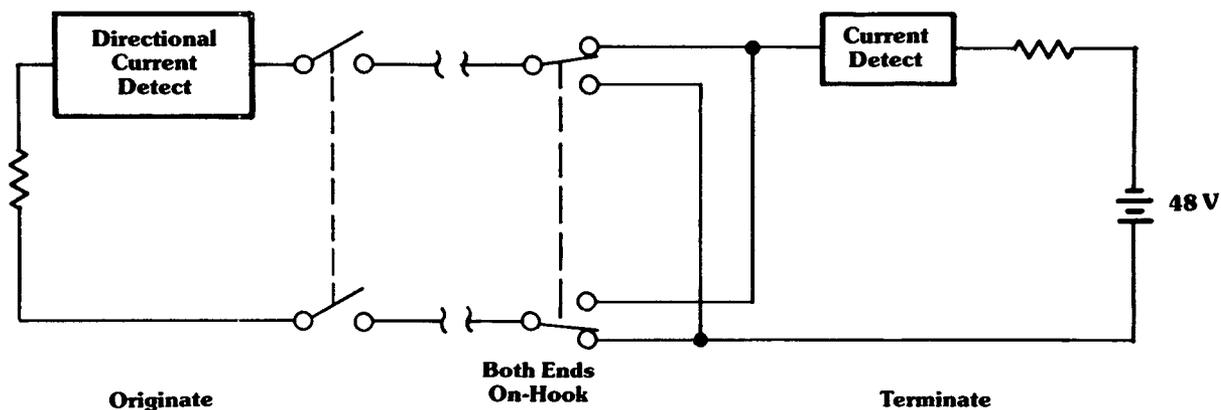
Figure 14. Loop reverse battery signaling.
