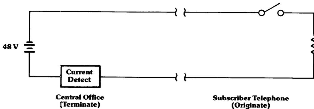
Figure 3. Loop signaling.
