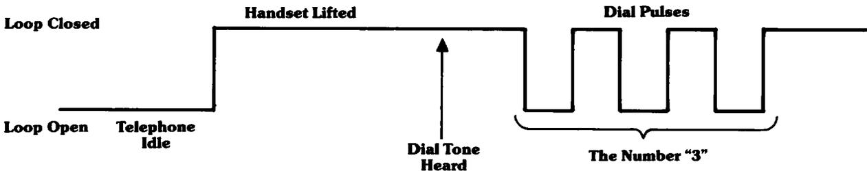
Figure 1. Telephone—off-hook and dial pulsing.
