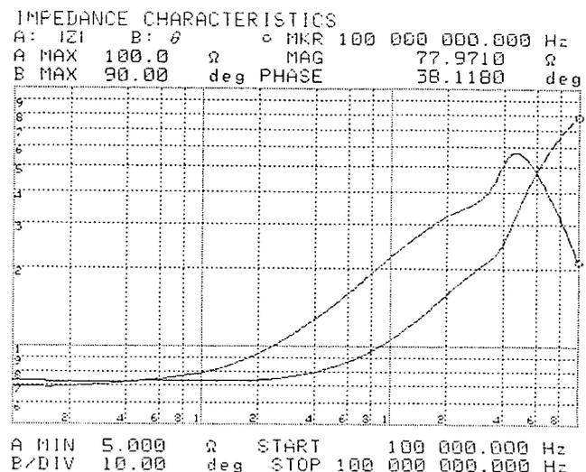
Figure 3. Output Impedance Characteristics
