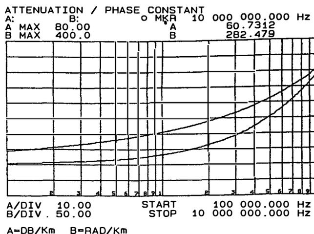
Figure 2 and 3 shows the results of a calculation using this ASP Program to evaluate the characteristic impedance and attenuation/phase constants of a twisted pair cable(170m long).
