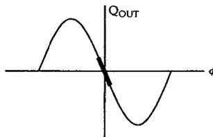
When  $\phi \approx 0$ ,  $Q_{out}$  is relatively insensitive to input amplitude fluctuations and relatively sensitive to phase fluctuations. The Q channel operates as a linear phase detector.
