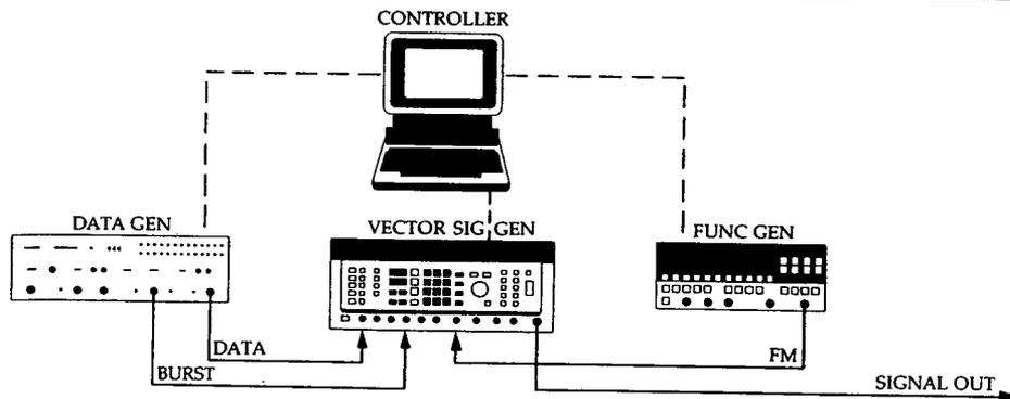
Figure 2b. This section of a vector measurement system generates complex modulated signals, including pulsed, phase coded, Barker coded, chirped, Doppler shifted, and many others.
