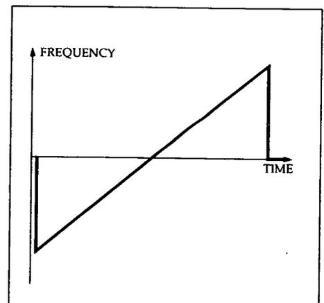
Figure 15. Plots related to the chirped signal in Figure 14. The frequency plot was calculated by taking the derivative of the phase plot. The phase plot was derived from I and Q.
