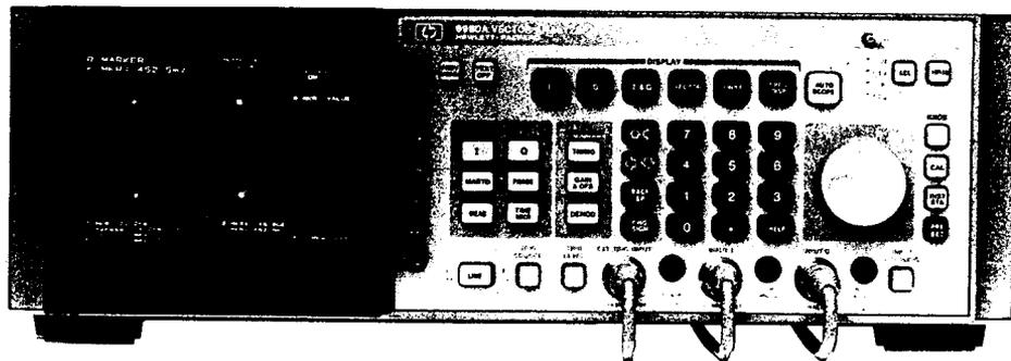
Figure 9. The front panel of the HP 8980A Vector Analyzer.
