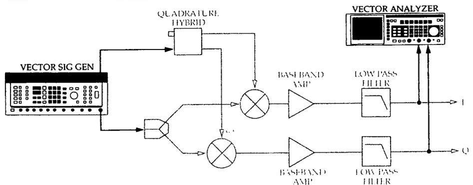
Figure 18. Calibrating a vector demodulator. The HP 8780A Vector Signal Generator inputs a test signal while the HP 8980A Vector Analyzer displays quadrature, gain, and dc errors. The demodulator can then be adjusted while watching the result on the vector display.
