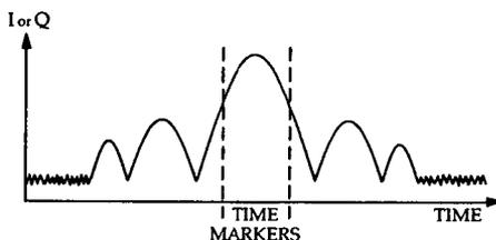
Figure 33. The output of a compressive receiver for a simple pulsed input.
