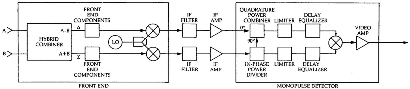
Figure 28. This monopulse receiver converts the amplitude measurement of the two channels into a phase measurement for processing.
