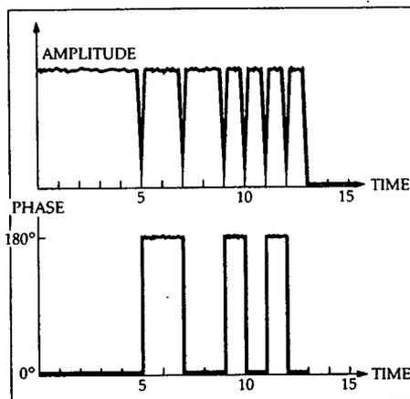
Figure 13. The phase and amplitude envelopes derived from I and Q channels of Figure 12. These plots show the phase code on the pulse.
