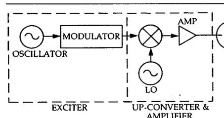
Figure 1. General modern transmitter block diagram. The modulation typically takes place before the power amplifier and at a lower frequency than RF. Older transmitters, tubes and cavity magnetrons would modulate at RF.
