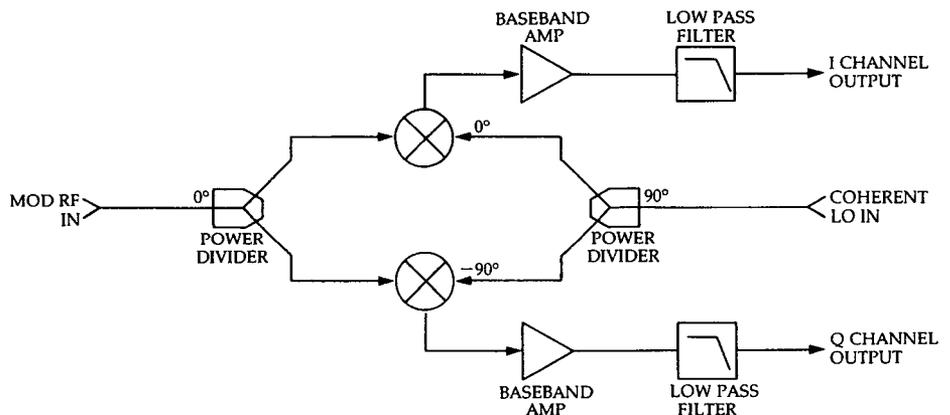
Figure 4. A vector demodulator reveals the phase between two inputs and the magnitude of the inputs. The phase, magnitude, and time information is contained on the two baseband output channels, I and Q.
