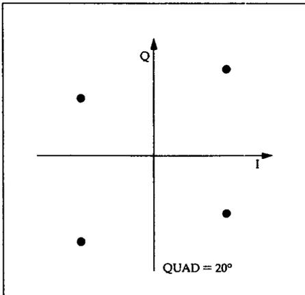
Figure 21. With both phase errors or both phase and gain errors in the demodulator, the QPSK signal appears as a parallelogram.
