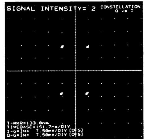
Figure 20. A QPSK signal will appear as a rectangle for gain mismatches in the I and Q channels.
