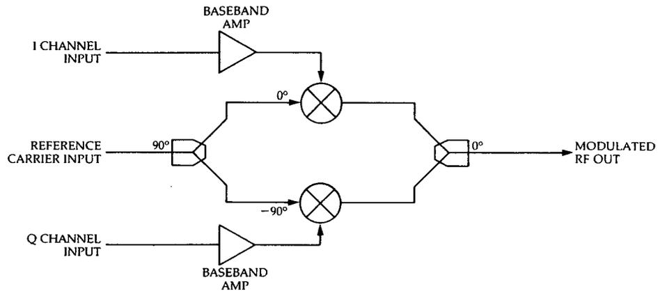
Figure 5a. A vector modulator synthesizes a complex modulated signal from baseband I and Q inputs and a CW carrier input.
