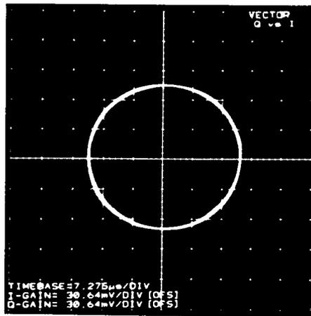
Figure 22. Vector diagram when a CW input to the demodulator has a frequency offset from the reference input. A constant frequency shift causes a constant phase change, which then plots a circle on the display. The display also represents a Doppler shifted return.
