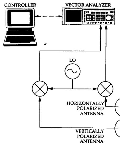
Figure 35. Displaying a signal's polarization with the HP 8980A Vector Analyzer.
