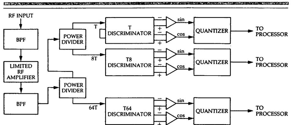
Figure 32. Digital instantaneous frequency measurement (DIFM) receiver.
