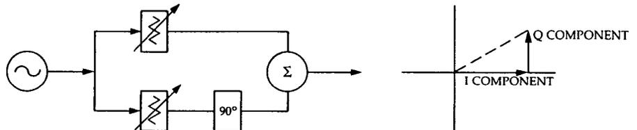
Figure 5b. Conceptual diagram of how a vector modulator operates. The incoming signal is split and passed through variable attenuators. One channel is given a  $90^\circ$  phase offset, then the two channels are summed. The two channels represent the quadrature components of the output signal. By varying the attenuation levels, the output phase and amplitude can be controlled.
