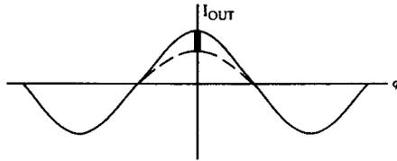
When  $\phi \approx 0$ ,  $I_{out}$  is relatively sensitive to input amplitude fluctuations and relatively insensitive to phase fluctuations. The I channel operates as a linear AM detector.
