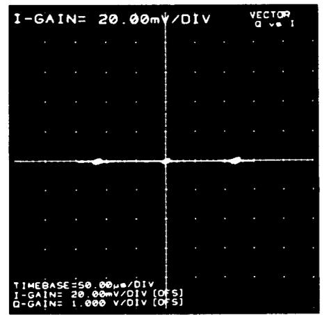
Figure 12. The vector diagram of a phase-coded pulse. The three states are displayed along with the trajectory paths taken between states. These paths indicate the signature of the radar.
