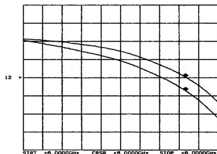
Figure J. Plot of a measurement of mixer conversion compression made using AC detection mode without and with the low-pass filter of Figure H (traces 1 and 2, respectively). No attenuation was used, in order to maximize the effect of the IF harmonics and feedthrough signals.
