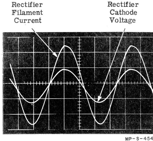
Figure 5. Waveforms Obtained With 154A
