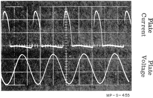
Figure 3. Waveforms Obtained With 154A
