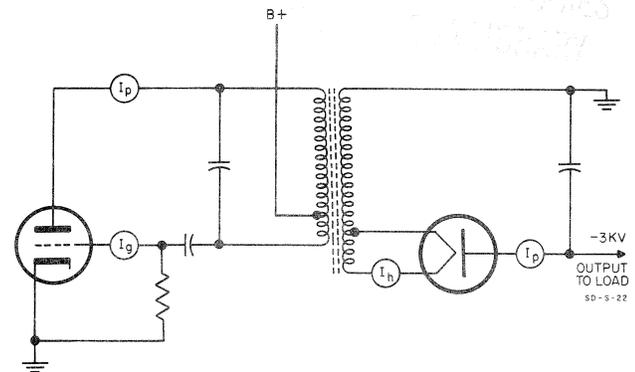
Figure 1. Typical RF Oscillator Used for an Oscilloscope Beam Supply
