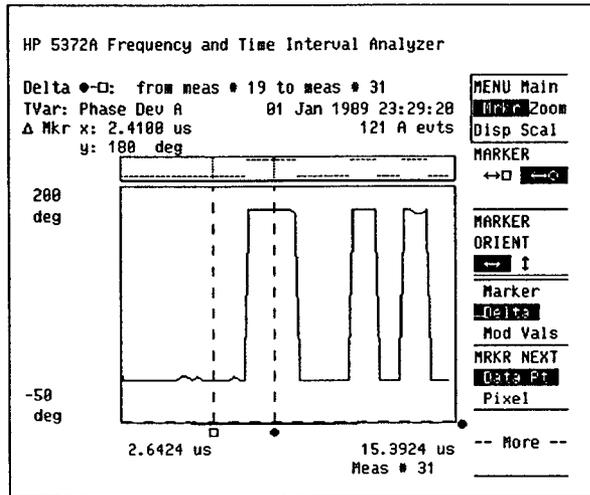
Figure 16. Using the markers to analyze a Barker modulated signal.
