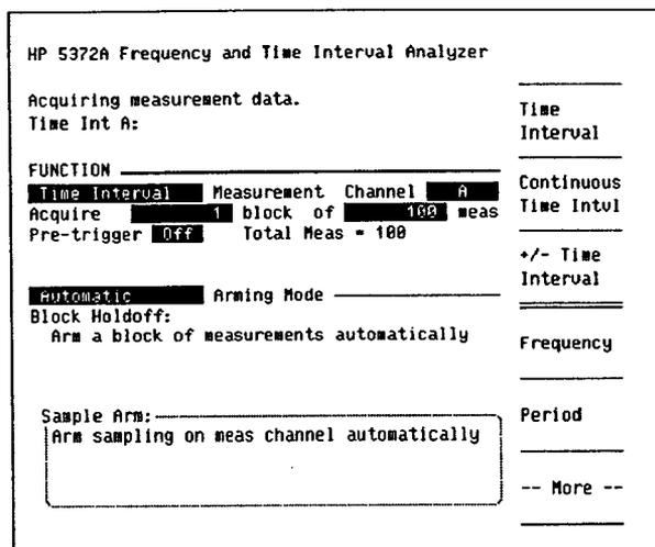
Figure 4. HP 5372A FUNCTION menu as it appears after pressing **Prset**.
