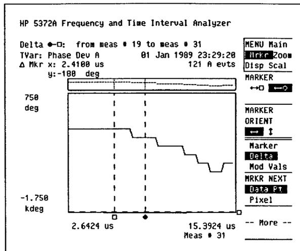
Figure 14. Using the markers in delta mode, you can determine the phase shift at each step in the code.
