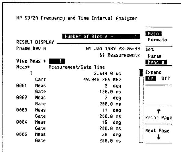
Figure 12. The numeric display is a list of phase measurement results. The “expanded” mode displays the carrier frequency used for the Phase Deviation measurement.
