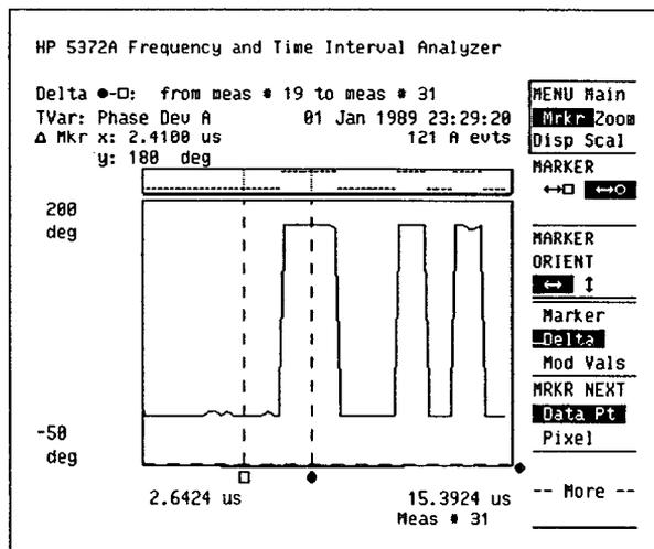
Figure 15. Phase deviation versus time using the Modulo 360 format shows the modulation in a more familiar form.
