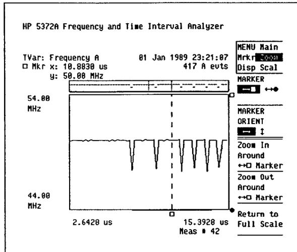
Figure 7. This plot of frequency versus time shows the effects of the Barker modulation.
