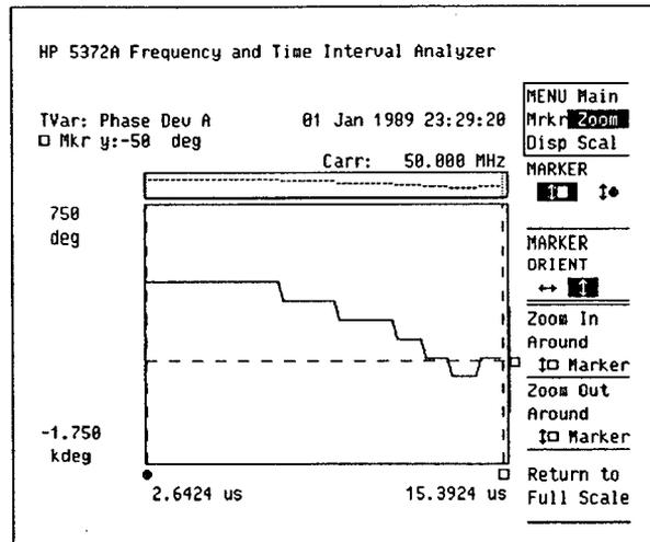
Figure 13. This plot of phase versus time shows the cumulative progression of phase through the Barker code
