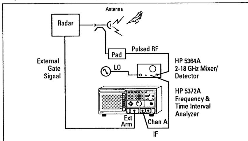
Figure 2. Typical equipment configuration for measuring Barker coded signals.
