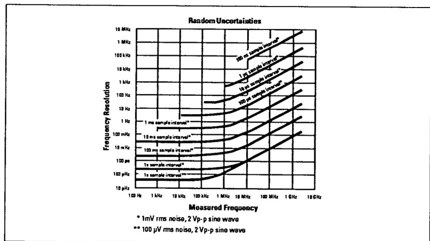
Figure 3. Frequency resolution depends primarily on sample interval and measured frequency.
