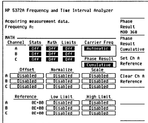
Figure 10. The **MATH** menu shows entries to compute the reference or carrier frequency automatically for Phase Deviation measurements. The results will be displayed as cumulative phase progression.
