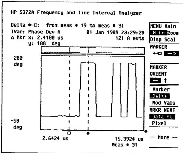
Figure 1. The HP 5372A lets you quickly and easily analyze complex radar signals, such as this 13 bit Barker modulated pulse.
