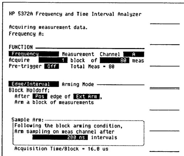
Figure 5. The completed **FUNCTION** menu shows selections for measurement type, number of measurements, arming, and sampling.
