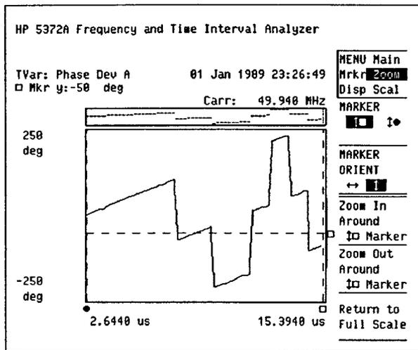
Figure 11. Example of Phase Deviation measurement with incorrect carrier frequency.
