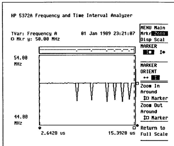
Figure 8. Positioning the [□] marker to estimate carrier frequency.
