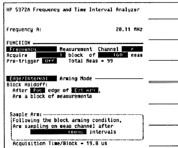
Figure 5. The completed **FUNCTION** menu shows selections for measurement type, block size, arming and sampling.
