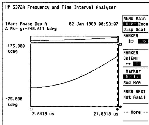
Figure 9. The phase deviation for a linear frequency chirp is a parabola.
