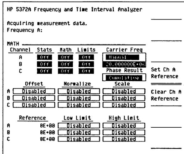
Figure 8. The MATH menu after entering carrier frequency and specifying type of phase display.
