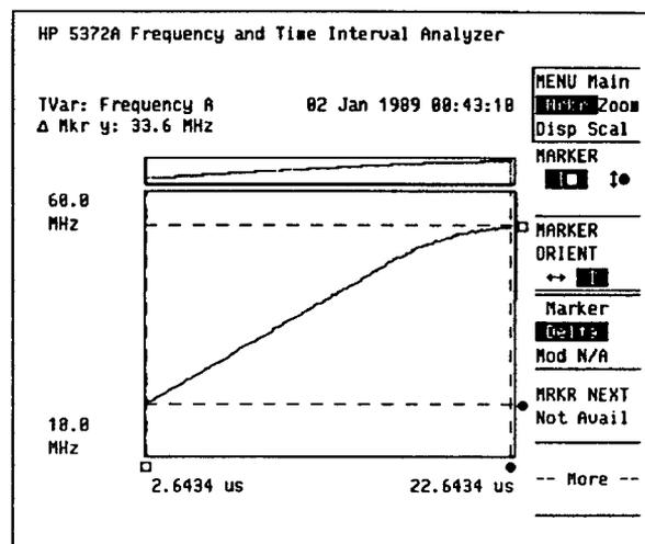
Figure 7. This plot of frequency versus time clearly shows the profile of a chirp which exhibits non-linear behavior.
