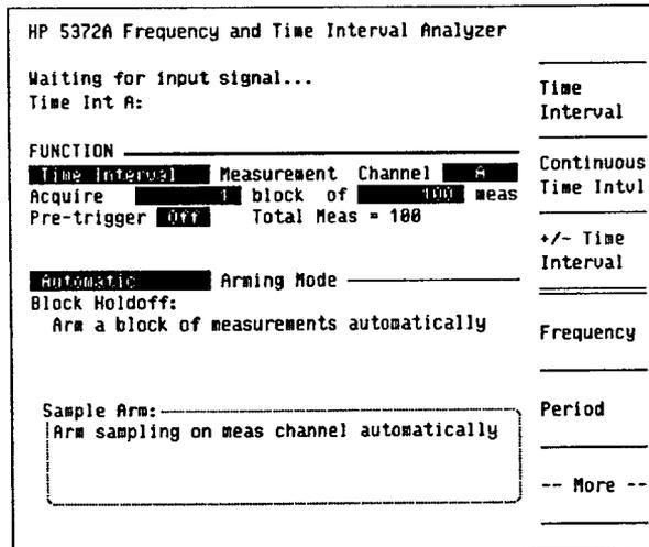
Figure 4. HP 5372A FUNCTION menu as it appears after pressing Preset.
