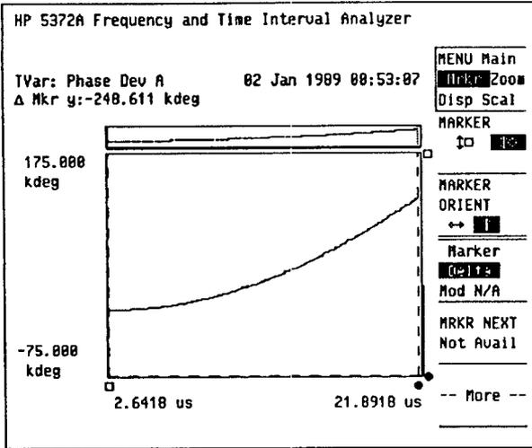
Figure 1. Phase as a function of time for a frequency-linear chirped radar pulse.
