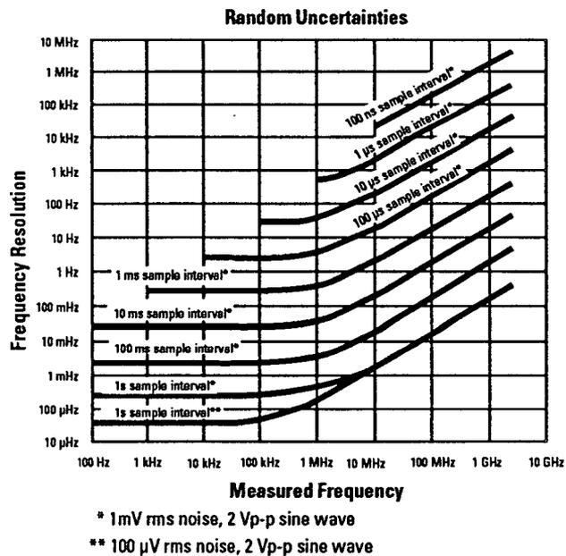
Figure 3. Frequency resolution depends primarily on sample interval and measured frequency.
