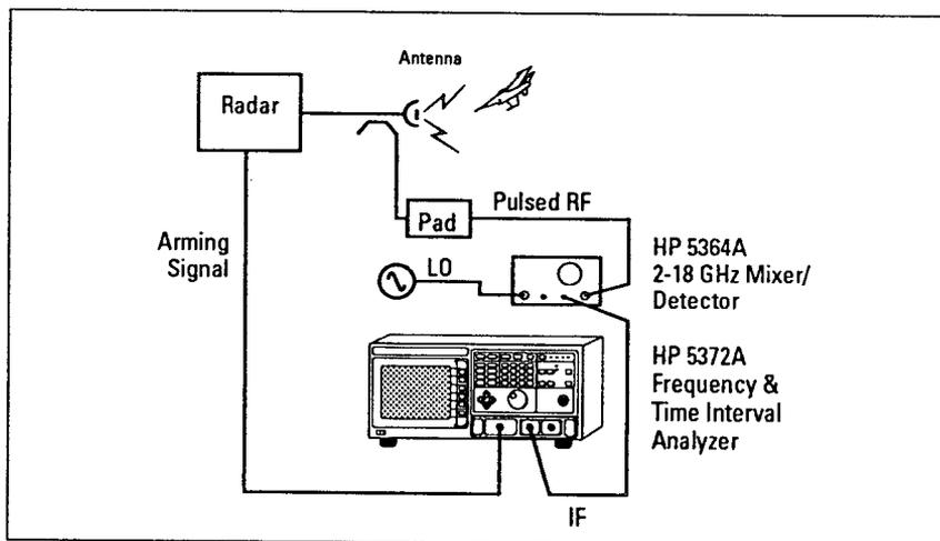
Figure 2. Typical equipment setup for measuring a chirped radar pulse.
