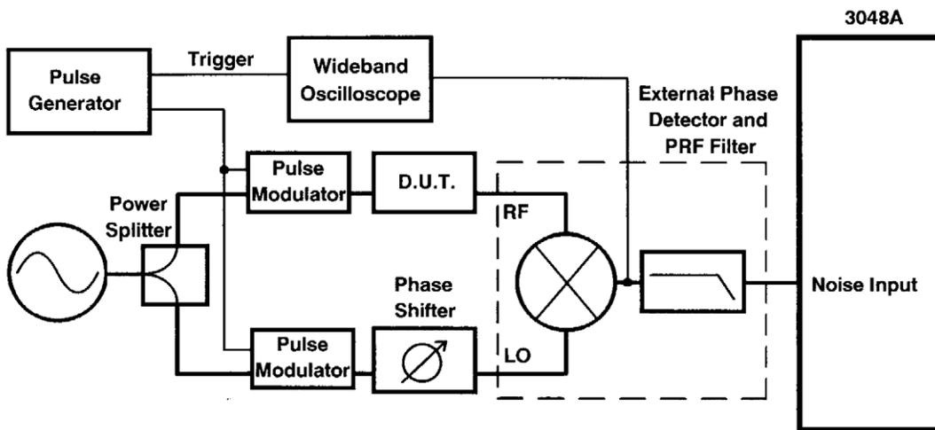
Figure 26. Recommended hardware configuration for making pulsed residual measurements when a PRF filter is required
