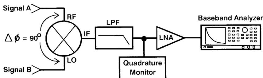
Figure 11. Block diagram of phase detector method of measuring SSB phase noise
