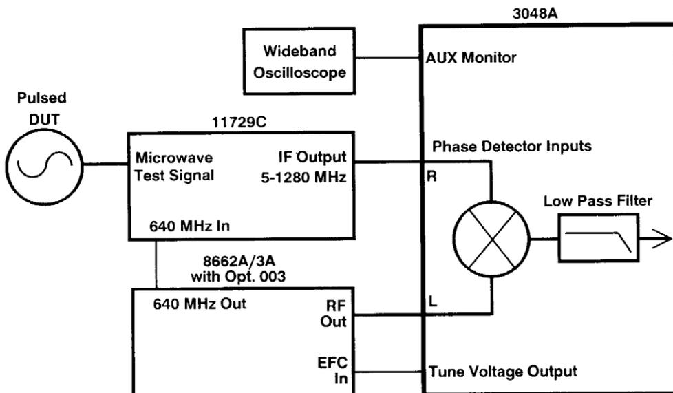
Figure 30. Recommended hardware configuration for making pulsed absolute measurements using the Agilent 3048A/11729C
