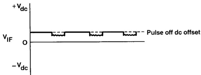
**Figure 17. Adjusting phase for minimum deviation from dc offset during pulse on period**
