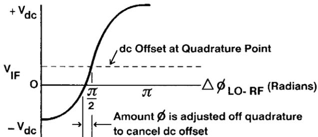
Figure 15. Cancelling dc offset by adjusting  $\Delta\Phi_{LO-RF}$  off quadrature
