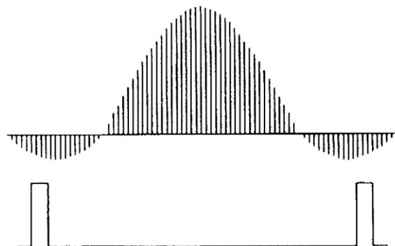
**Figure 5c. PRF lower than 5a results in higher spectral density. Lobe width is same as 5a since pulse widths are identical.**
