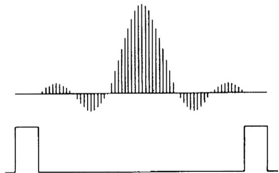
**Figure 5d. Spectral density and PRF unchanged from 5c but lobe widths are reduced by wider pulse.**
