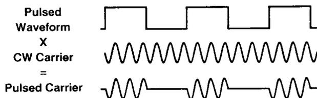
Figure 7. Multiplication of a CW carrier by a pulsed waveform results in a pulsed carrier.
