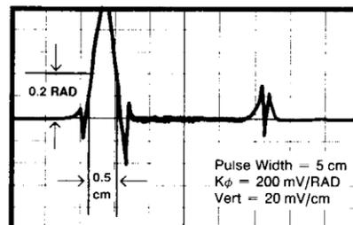
**Figure 23.** Phase transients exceeding 0.2 radians for more than 10% of pulse width as observed on oscilloscope connected to AUX monitor port
