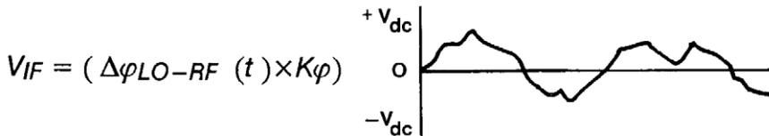
Figure 12. Phase detector output for a CW signal
