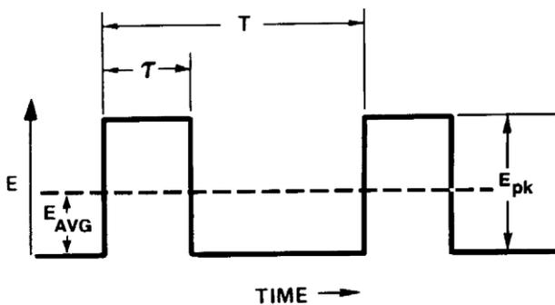
**Figure 3. Basic characteristics of a pulsed waveform**
