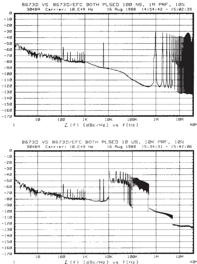
Figure 31. Pulsed synthesizer absolute phase noise plots
