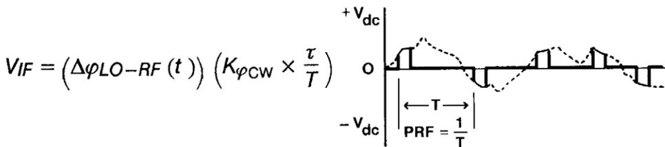
Figure 13. Phase detector output for a pulsed carrier
