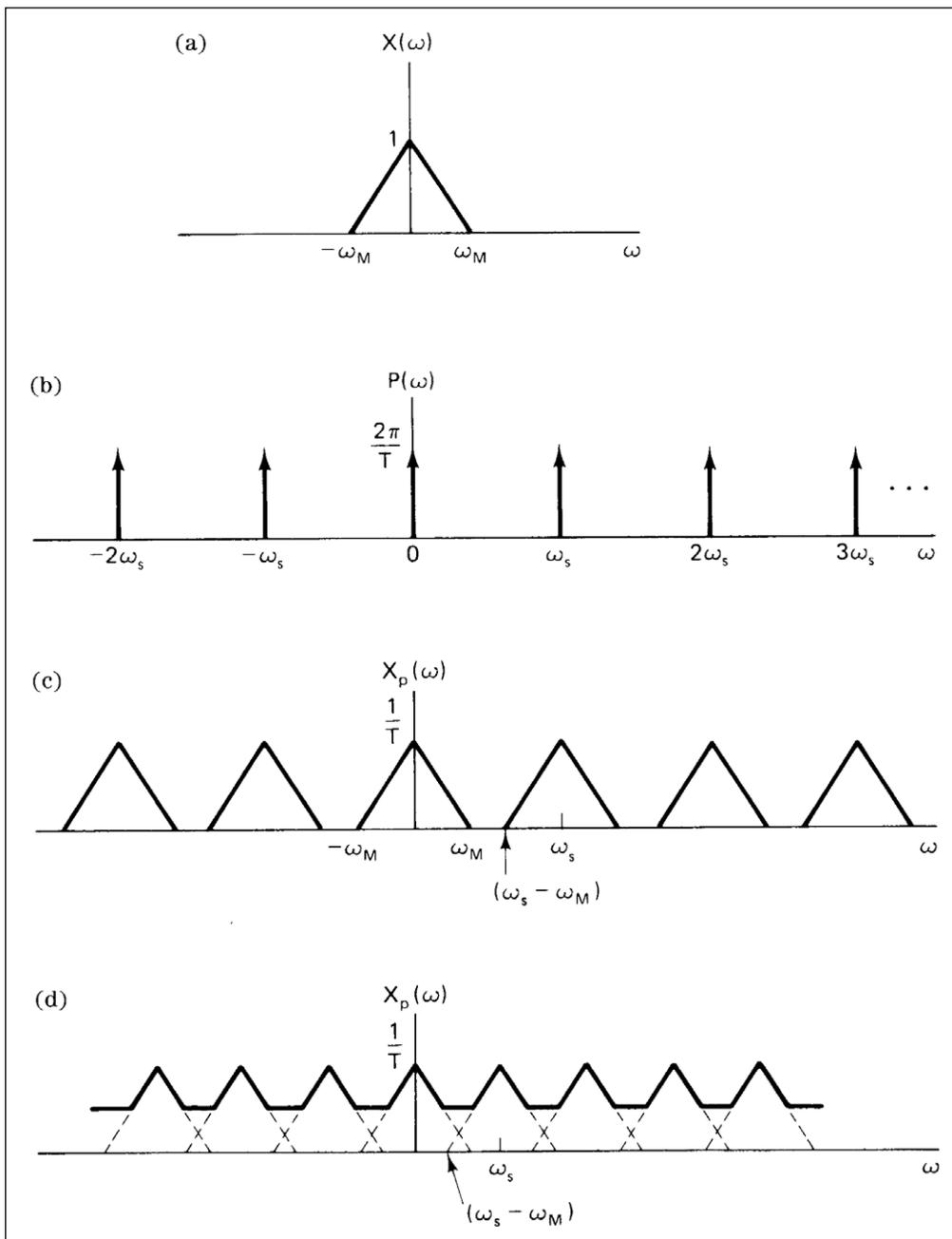
**Figure 14. Effect in the frequency domain of sampling in the time domain**
