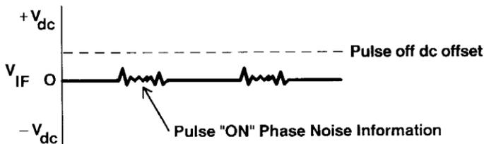
Figure 20. Phase detector output, at quadrature, when pulsing both inputs
