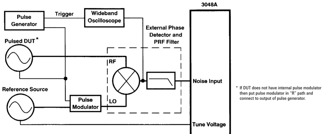
Figure 27. Recommended hardware configuration for making pulsed absolute measurements when a PRF filter is required
