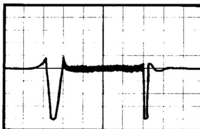
**Figure 22.** Phase transients with saturation as observed on oscilloscope connected to AUX monitor port
