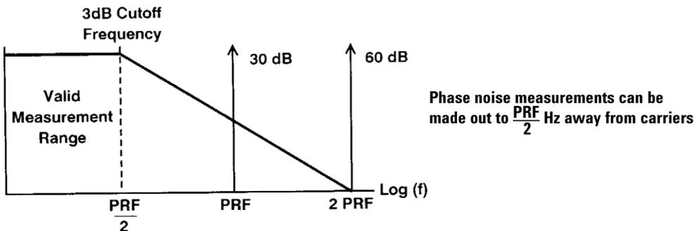
Figure 25. PRF filter response characteristics
