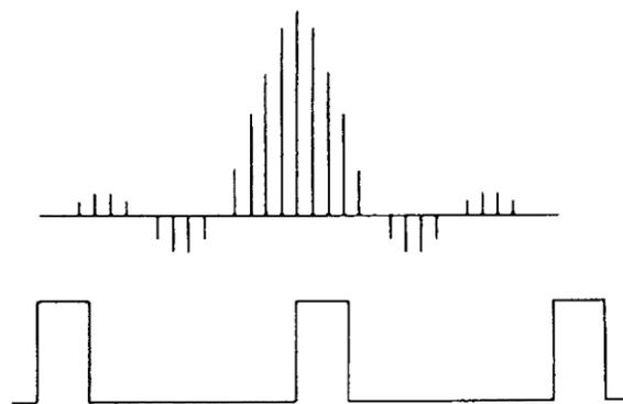
**Figure 5b. Wider pulse than 5a causes narrower lobes, but line density remains constant since PRF is unchanged.**
