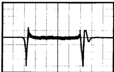
**Figure 21.** Phase transients at output of phase detector as observed on oscilloscope connected to the AUX monitor port
