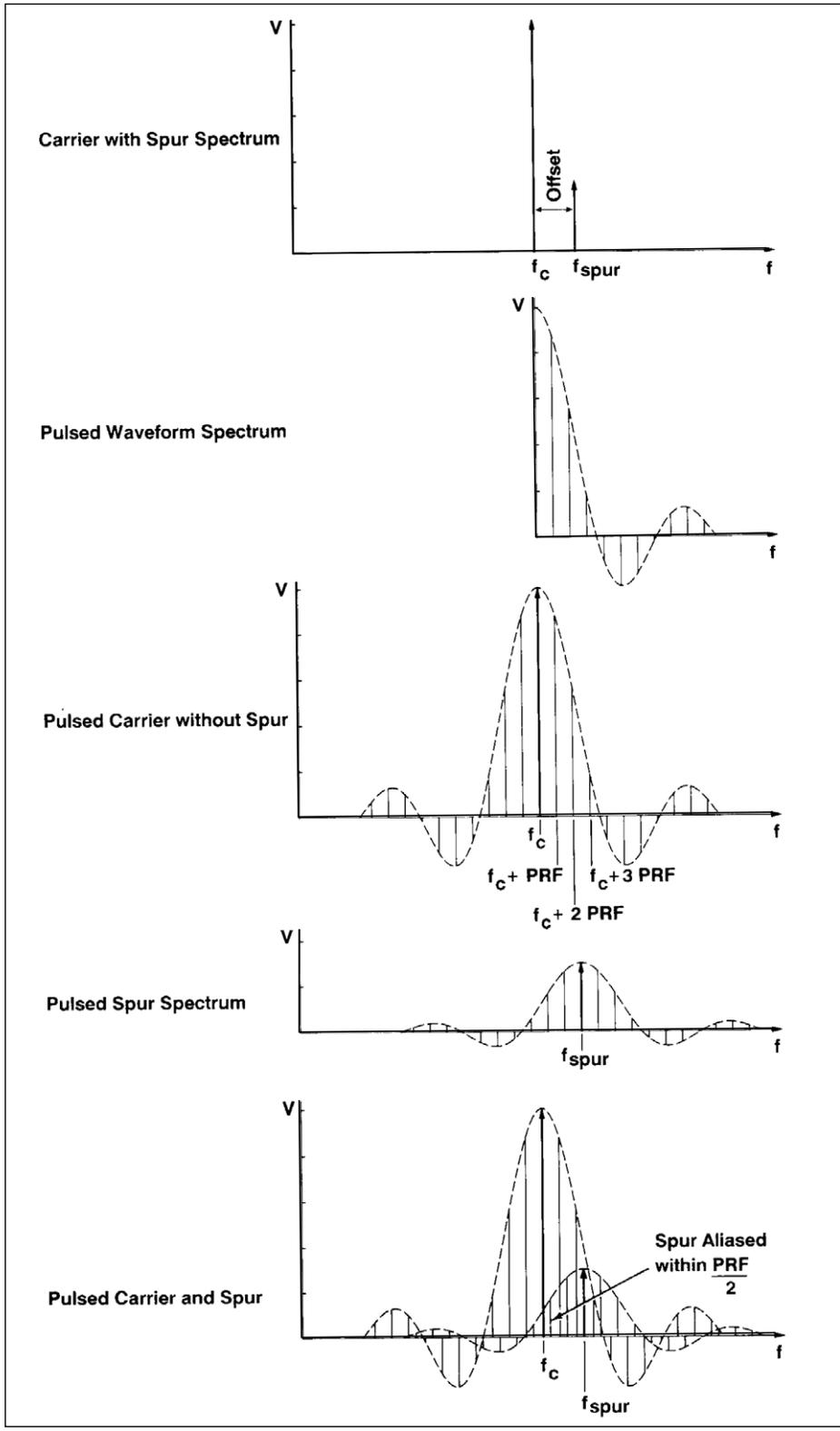
Figure 9. Convolution of a CW carrier with spur spectra and a pulsed waveform spectra
