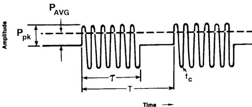
Figure 6. Basic characteristics of a pulsed carrier
