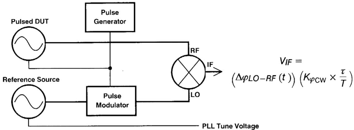
Figure 19. Recommended configuration for making pulsed absolute noise measurement
