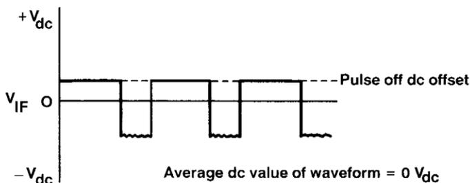
Figure 16. Compensating for dc offset by adjusting  $\Delta\Phi_{LO-RF}$  to produce an average dc value of 0 Vdc
