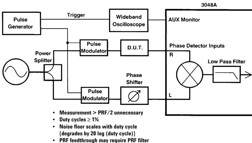
Figure 28. Recommended hardware configuration for making pulsed residual measurements using the Agilent 3048A
