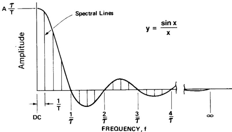
**Figure 2. Spectrum of a perfectly rectangular pulse. Amplitudes and phases of an infinite number of harmonics are plotted, resulting in a smooth envelope as shown.**
