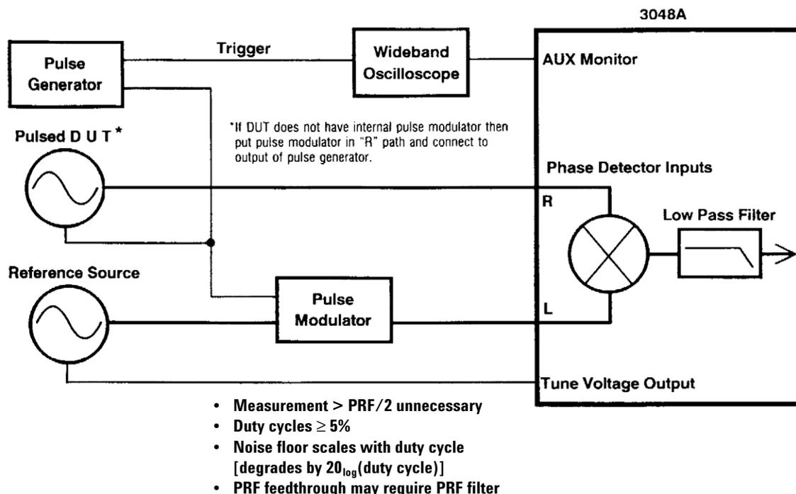
Figure 29. Recommended hardware configuration for making pulsed absolute measurements using the Agilent 3048A
