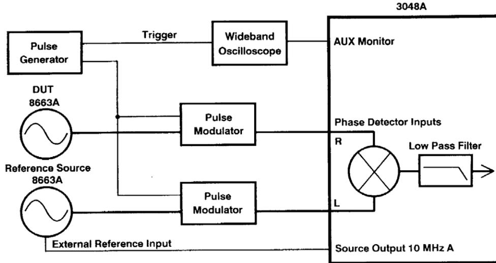
**Example 1: Agilent 8663A versus 8663A Pulsed Source Measurement**
