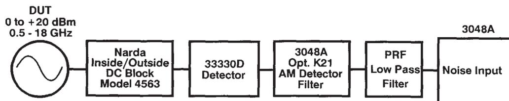
Figure 32. Recommended hardware configuration for making pulsed AM noise measurements using the Agilent 3048A
