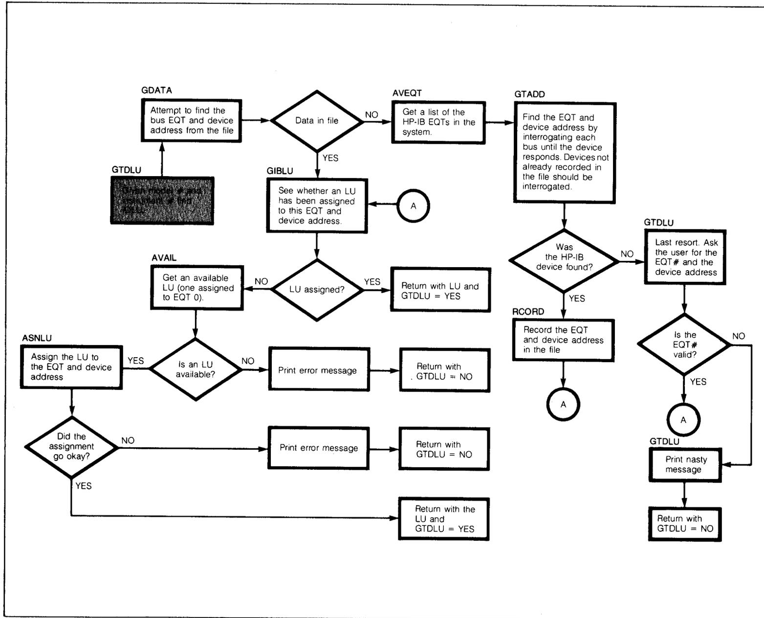
Figure 6-5. Flowchart Showing the Steps Required for HP-IB LU Determination Using GTDLU
