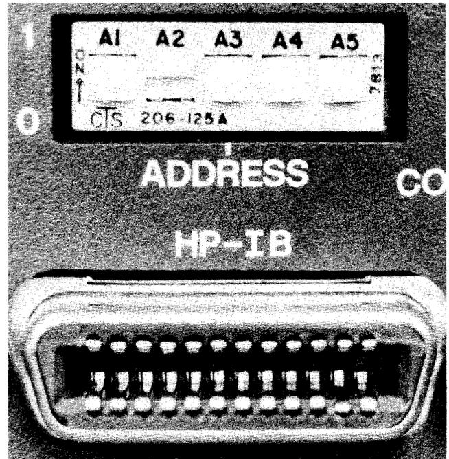
**Figure 1-4. A Typical Set of Address Switches**
