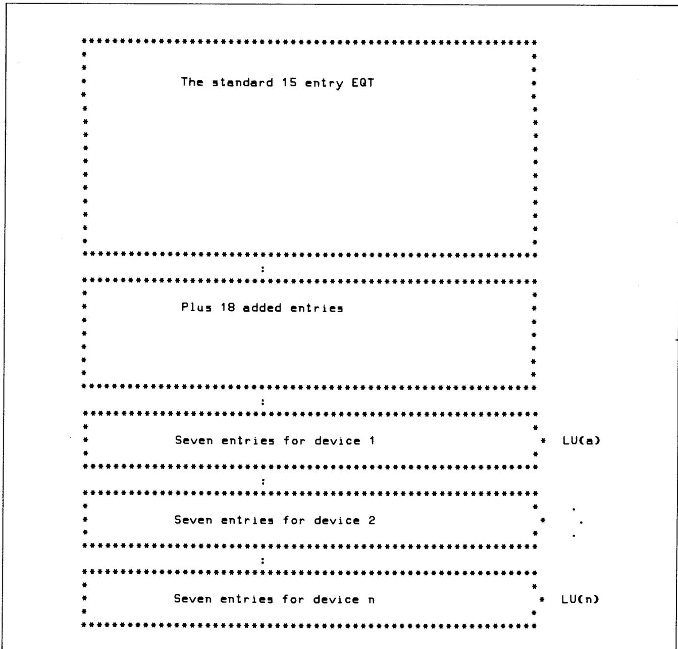
Figure 3-1. Extension of the Original EQT for HP-IB
