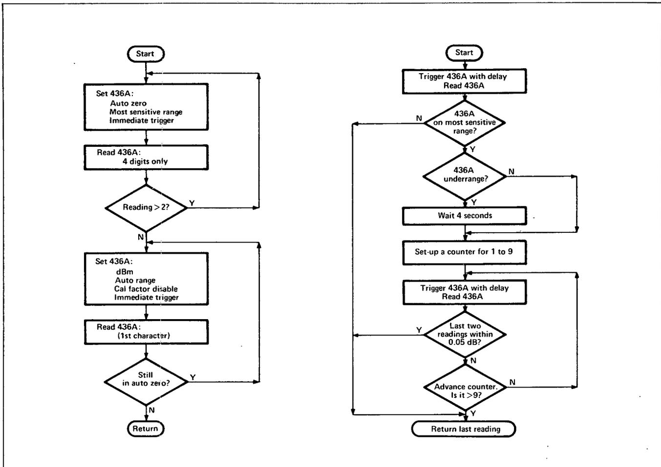
Figure 16-5. Flowchart for 436A Device Subroutines
