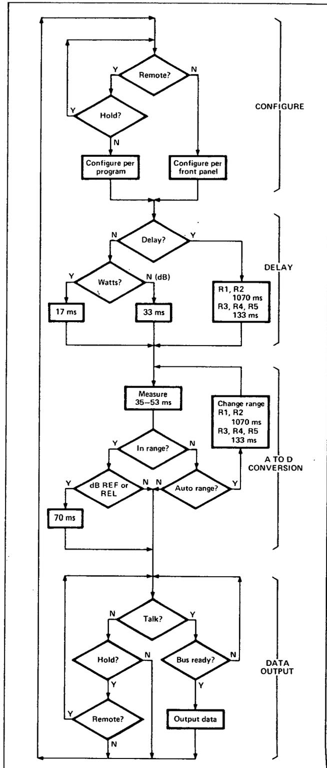
Figure 16-7. Flowchart for 436A Internal Timing
