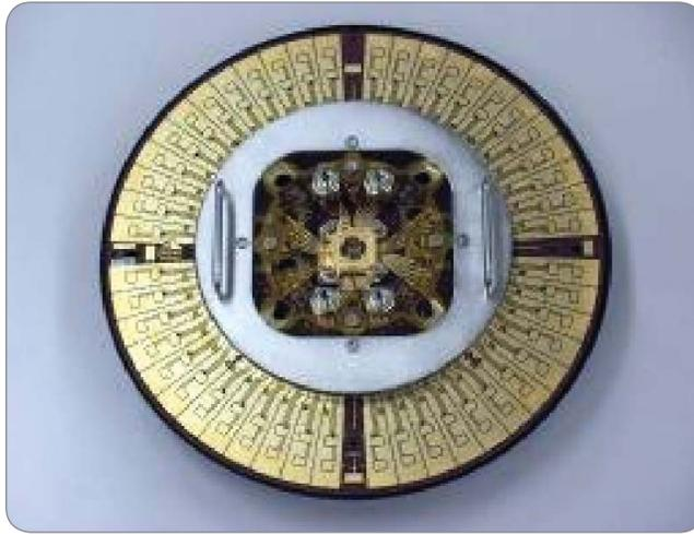
Figure 6a. The Cascade Microtech, Inc. Pyramid Probe card for the 4083A RF docking interface
