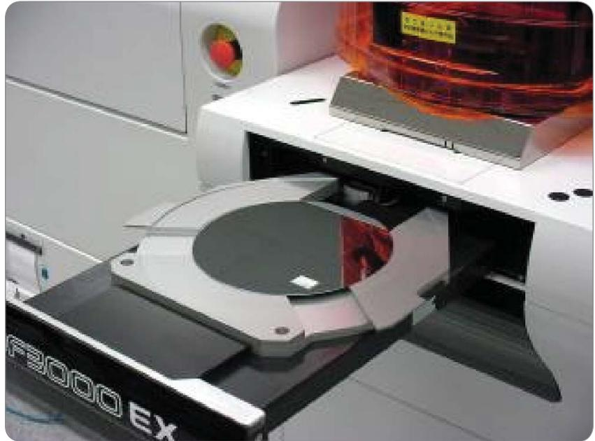
Figure 5a. Using an impedance standard substrate (ISS) on an adapter disk in an automated wafer prober.
