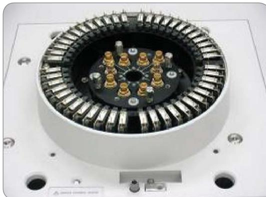
Figure 1a. The 4083A RF docking interface
