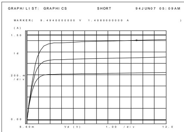
Figure 5. Example of Drain Characteristic Measurements
