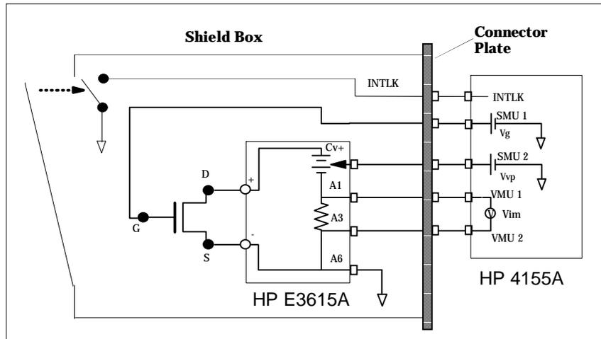
Figure 1. Diagram of Connections for Power Transistor Measurement
