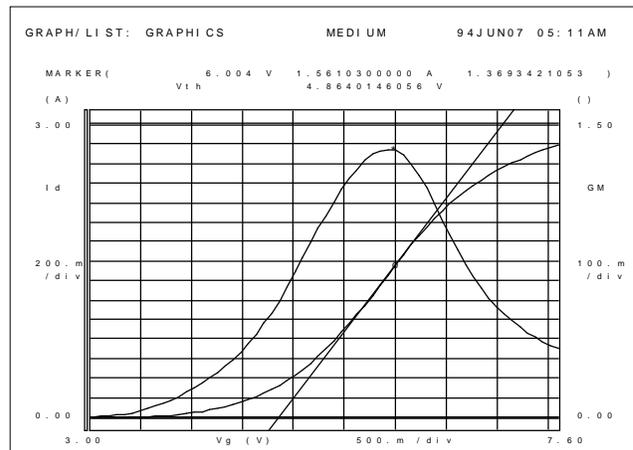
Figure 6. Drain Current versus Gate Voltage Characteristics to Obtain Vth
