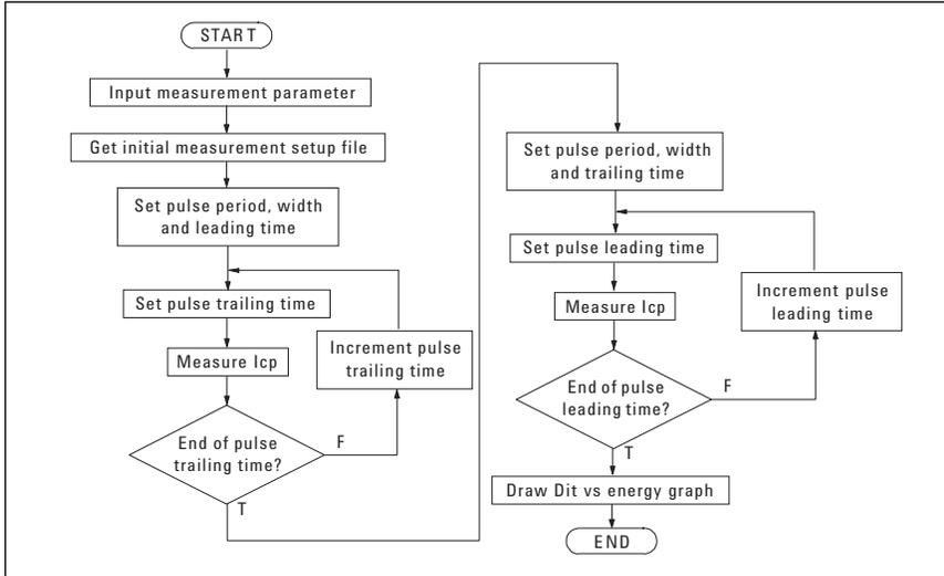
**Figure 14. Flowchart of Trapezoidal Pulse Method**
