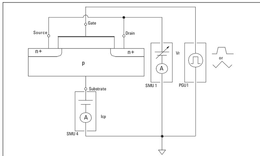
Figure 1. Measurement Circuit Diagram
