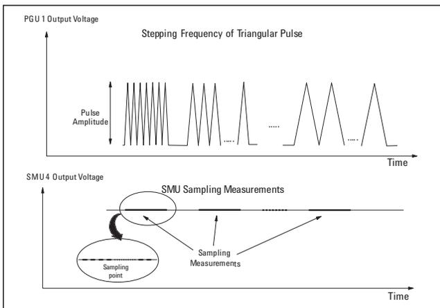
Figure 10. Timing Chart of Triangle Pulse Method
