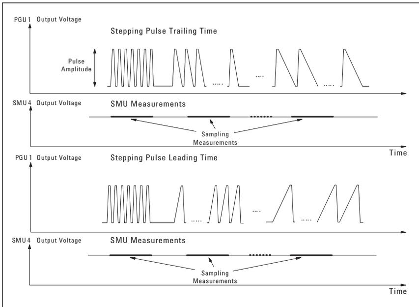
**Figure 15. Timing Chart of Trapezoidal Pulse Method**
