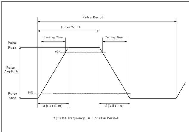
Figure 6. Definition of Square Pulse Setup Parameters
