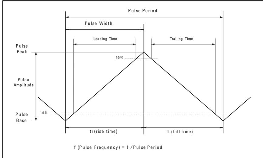
Figure 12. Definition of Triangle Pulse Setup Parameters
