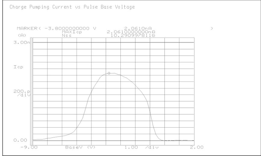
Figure 8. Square Pulse Method Nss Measurement Result
