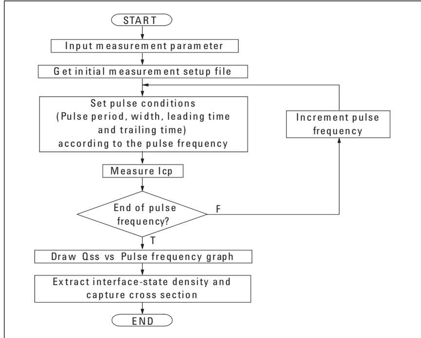
Figure 9. Flowchart of Triangle Pulse Method
