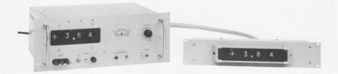
There are numerous applications where a remote indication of the voltage readings of the Model 405AR Digital Voltmeter is desirable or necessary.
