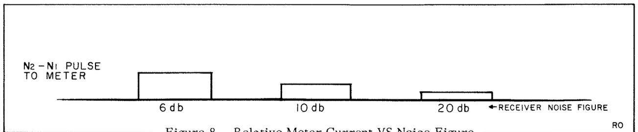
Figure 8. Relative Meter Current VS Noise Figure
