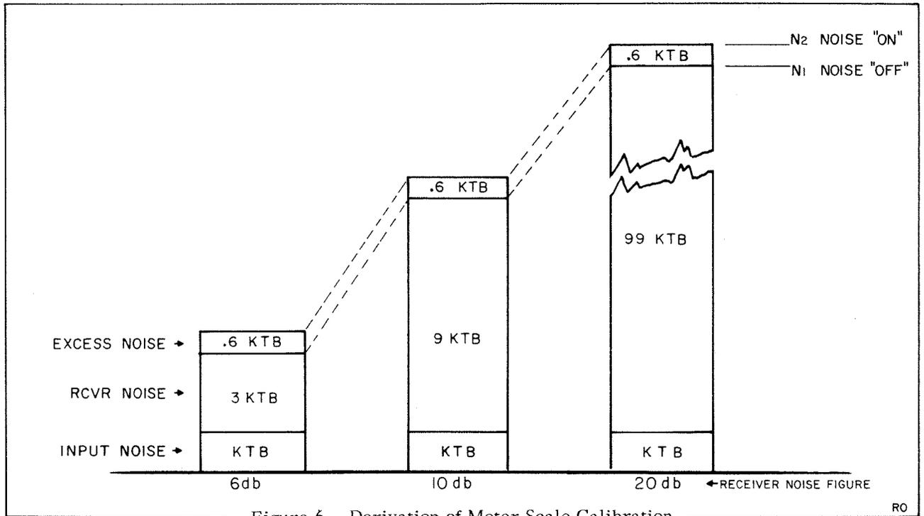
Figure 6. Derivation of Meter Scale Calibration
