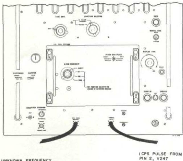
Figure 1. Using the 526C Period Multiplier Unit to Provide Longer Gate Times for the 524C/D Electronic Counters
