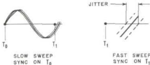
Figure 8. Jitter Measurement
