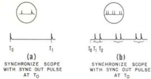
Figure 6. Sweep Calibration
