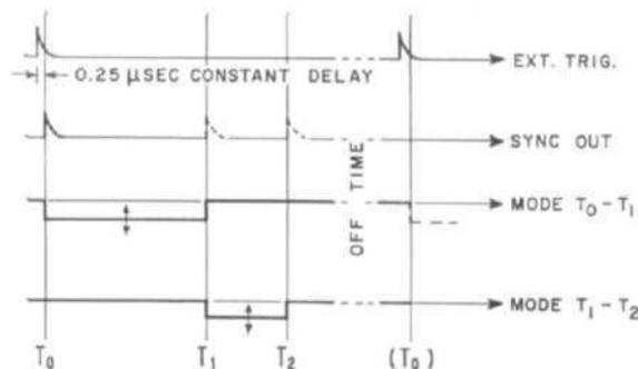
Figure 3. Time Plan, 219C Plug-In Unit
