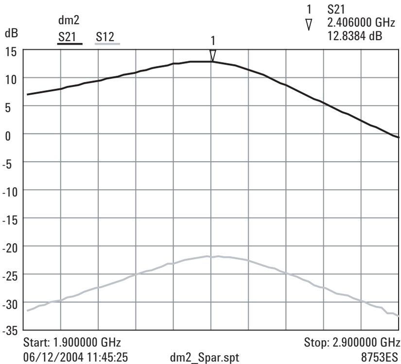
Figure 11. Measured forward gain and reverse isolation
