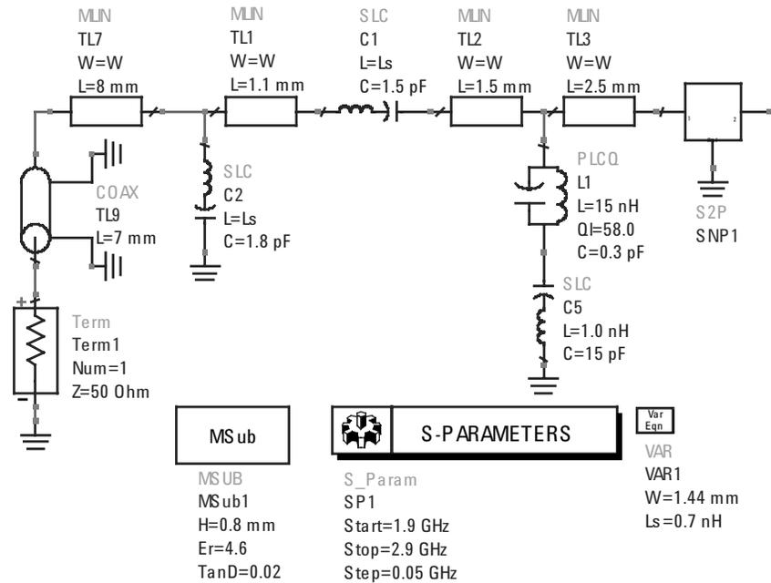
Figure 5. Input matching & biasing networks
