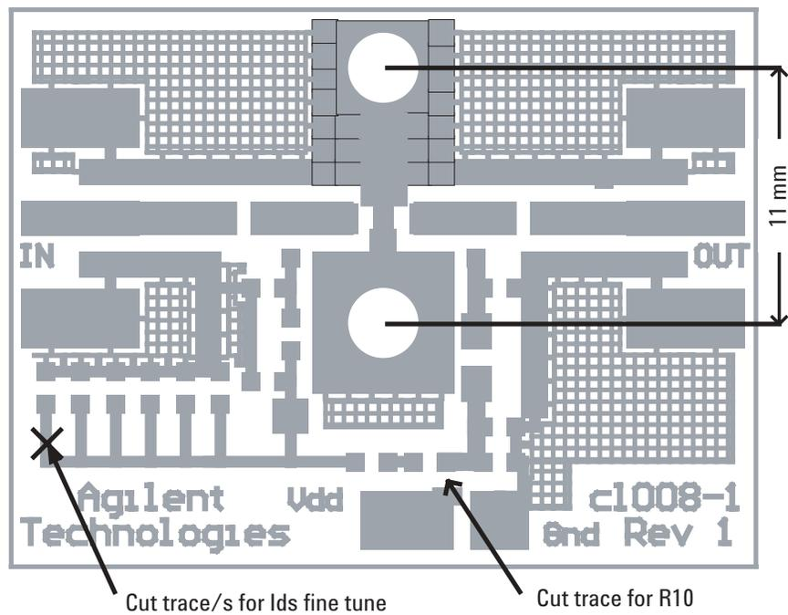
**Figure 4. Positions of PCB trace cuts and distance between heatsink screws**
