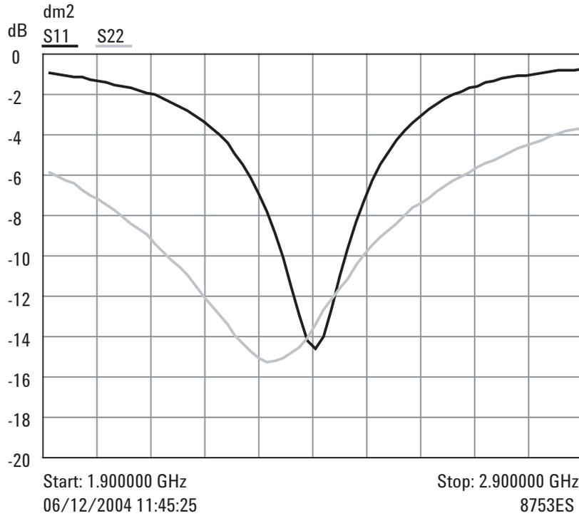
Figure 10. Measured input and output return loss
