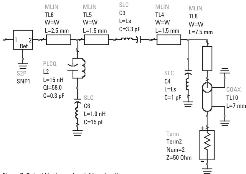
Figure 7. Output biasing and matching circuit
