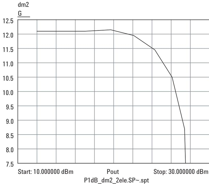
Figure 12. Measured gain vs. output power
