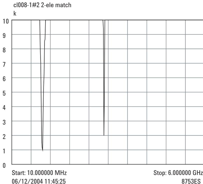
Figure 14. Stability ( $k$ ) calculated from measured s-parameters
