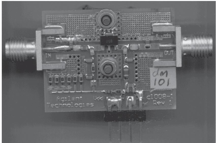
Figure 2. Fully assembled demoboard with connectors and screws for heatsink
