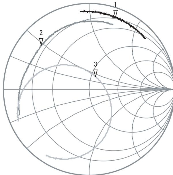
Figure 6. Measured trajectories of input impedance during the various phases of matching
