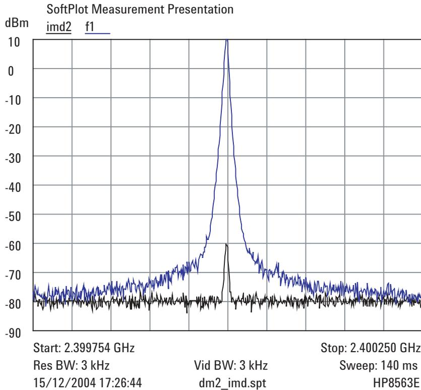
Figure 13. Overlay of fundamental tone and intermodulation product
