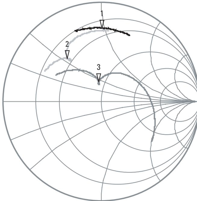
Figure 8. Measured trajectories of output impedance
