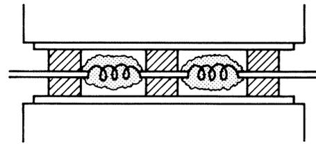
(c) INDUCTORS COATED WITH THIN LAYER OF POLYIRON
