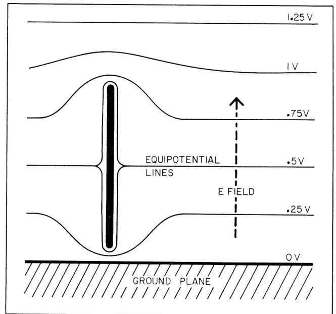
Figure 6. Derivation of Antenna Factor for 1 Meter Rod
