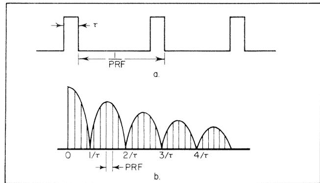
Figure 10. Pulse Spectrum
