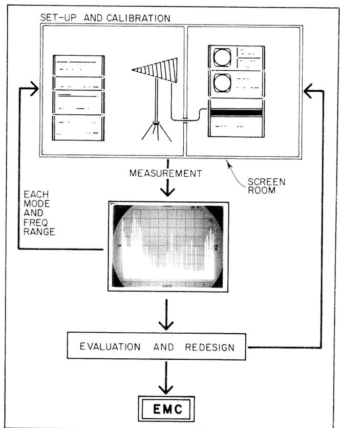
Figure 3. EMI Measurement Flow Chart
