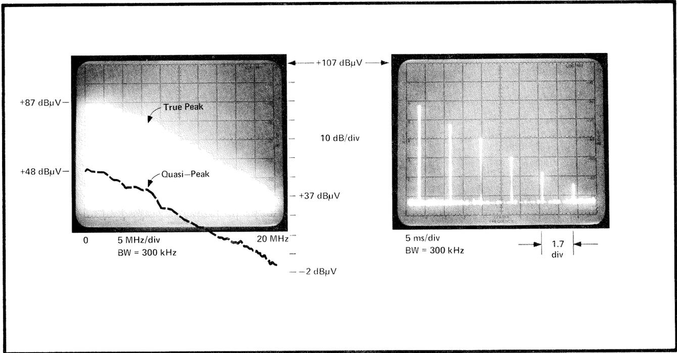
**FIGURE 1.** (a) This is the true peak of conducted EMI from an SCR light dimmer, and the quasi-peak level found from the graph. (b) The PRF is determined by video triggering and using the calibrated scan time to determine the time between pulses.
