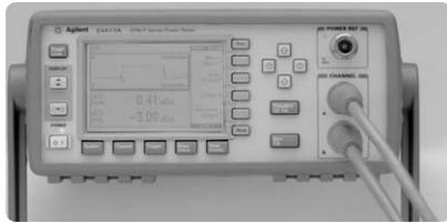
Figure 11. E4417A power meter configured to show a trace display (upper window) and a dual numeric display (lower window).
