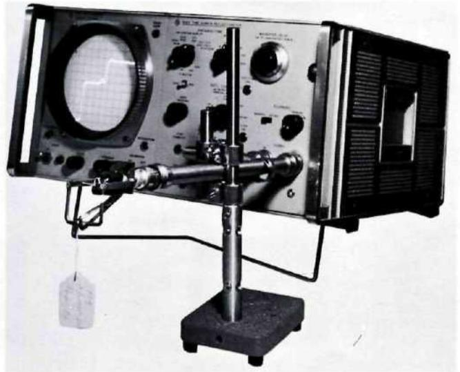
Figure 13. TDR Test of Transformer Subassembly
