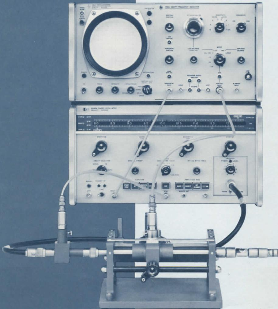
*An important new swept-frequency technique permits quick and accurate measurements of SWR in coaxial systems up to 18 GHz.*
