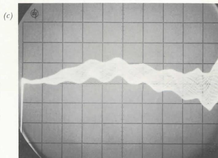
Fig. 2. Oscillograms made with setup of Fig. 1, showing measurement of SWR of a load.
