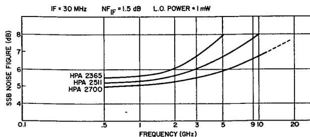
Figure 17. Typical Noise Figure vs. Frequency  $P_{LO} = 1$  mW.  $f_{IF} = 30$  MHz.  $NF_{IF} = 1.5$  dB
