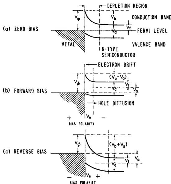
**Figure 3.** Energy Level Diagram for Hot Carrier Diode
