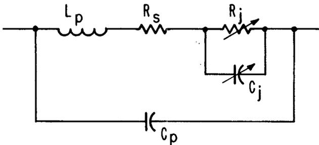
Figure 4. Equivalent Circuit of Hot Carrier Diode
