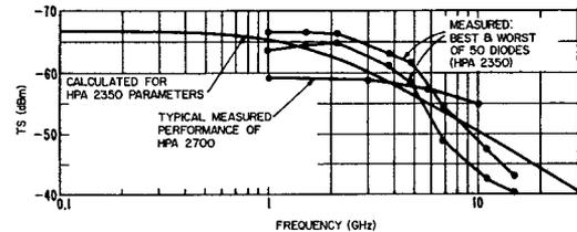
Figure 15. Tangential Sensitivity of Hot Carrier Diode
