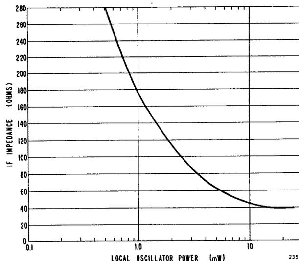
Figure 10. IF Impedance of HPA 2350 Hot Carrier Diode
