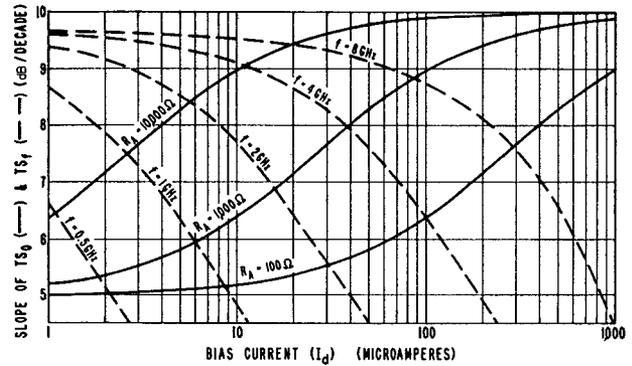
Figure 14. Optimum Bias for Specified Frequency (f) and Amplifier Noise Resistance ( $R_A$ )
