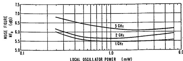
Figure 16. Typical Noise Figure vs. Local Oscillator Power (HPA 2350)  $f_{IF} = 30$  MHz.  $NF_{IF} = 1.5$  dB
