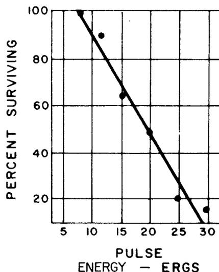
Figure 6. Burnout Resistance of Hot Carrier Diodes
