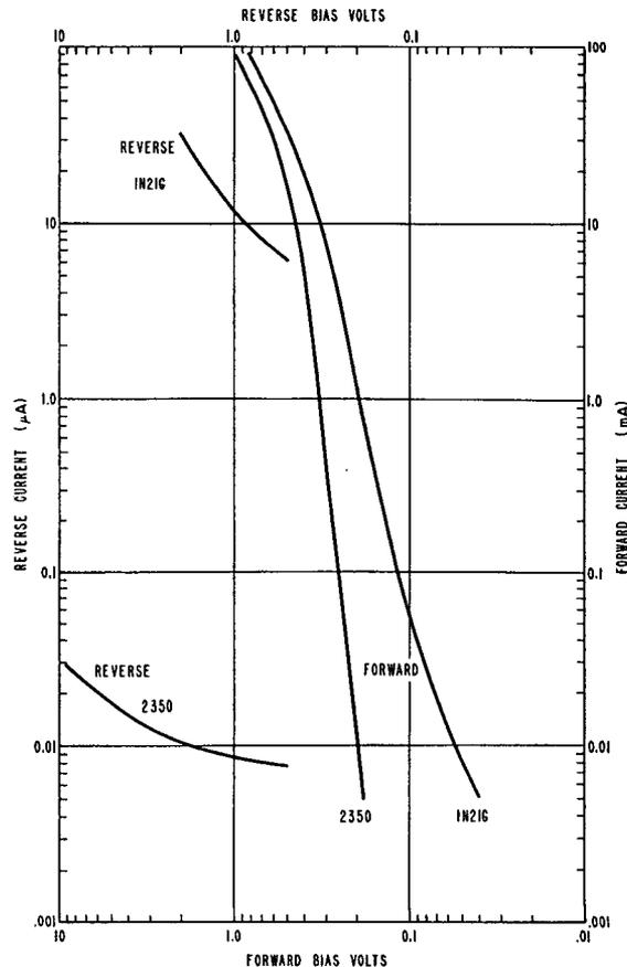
Figure 9. Forward VI Characteristics
