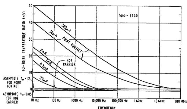
Figure 7. Noise Characteristics of Hot Carrier Diode
