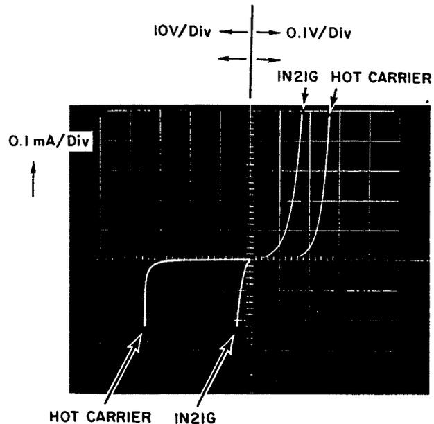
Figure 2. VI Characteristics of Hot Carrier and Point Contact Diodes
