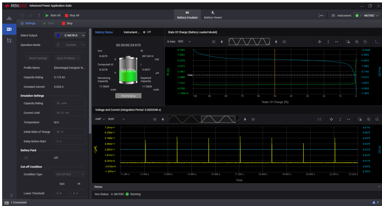
Figure 8.10. Using a battery model created using the Profiler feature, you can emulate the behavior of the battery at any desired state-of-charge within a matter of seconds
