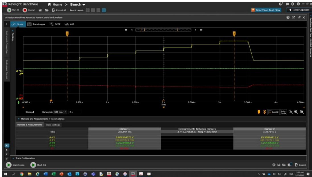
Figure 6.02. DC to DC converter efficiency test example.
