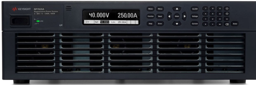
Figure A.09. The RP7900 regenerative power system returns sunk power to the AC line, thereby saving power and reducing dissipated heat.
