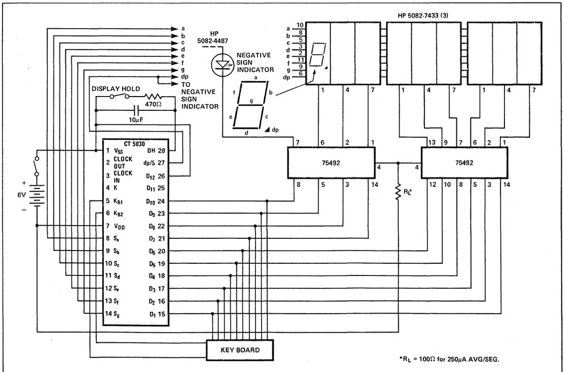
Figure 5. Four Function Calculator.
