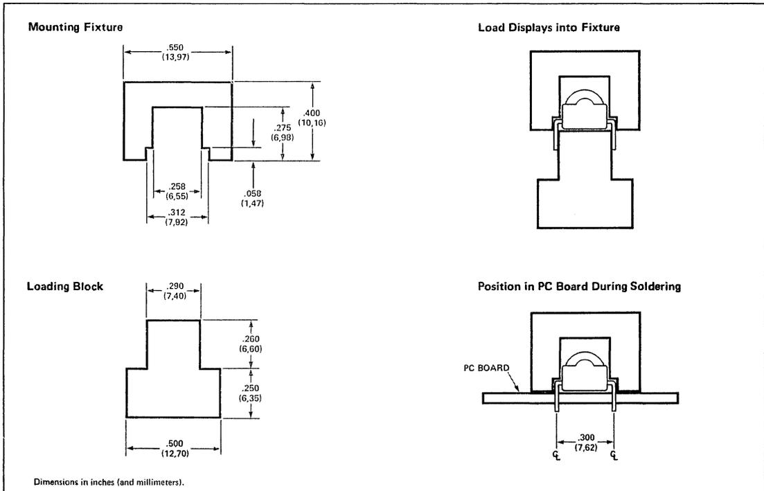
Figure 6. Mounting Fixture.
