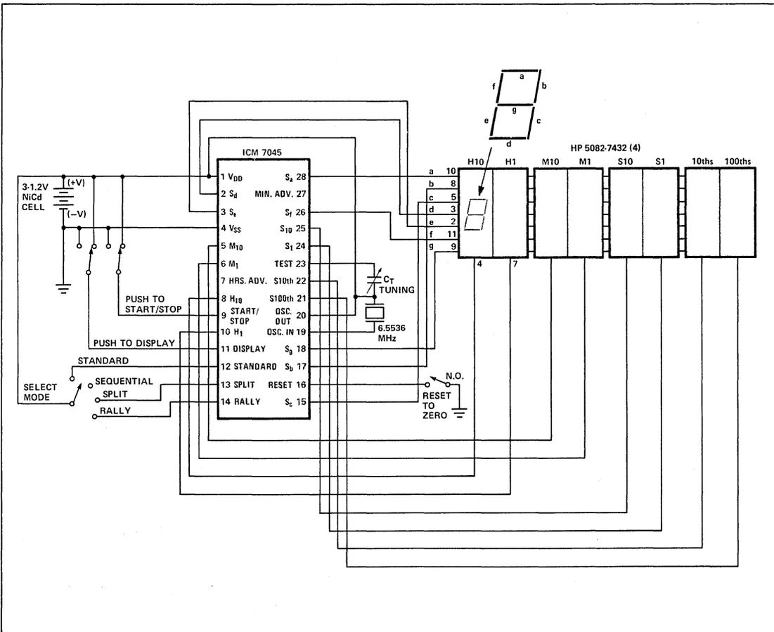
Figure 3. Electronic Stopwatch.
