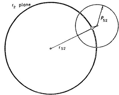
Fig. 3 — Circle defined by \$r\_{s2}\$ and \$\rho\_{s2}\$ divides \$r\_2\$ plane into a stable and potentially unstable region of operation. If \$|s\_{11}| < 1\$, the inside of the circle indicates those loads which provide negative real input impedance (\$|s\_{11}'| > 1\$). The heavier weight circle defines the unit circle on the Smith Chart.
