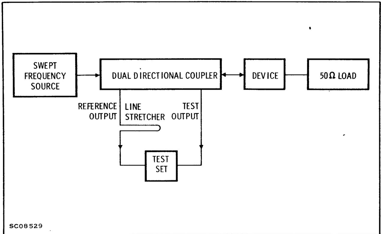
Figure 3. Setup for Measuring  $S_{11}$  and  $S_{22}$
