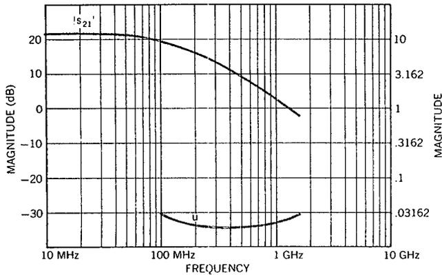
Fig. 5. Top curve:  $|s_{21}|$  from Fig. 4 replotted on logarithmic frequency scale. Data below 100 MHz measured with  $\sim$ hp-8405A Vector Voltmeter. Bottom curve: unilateral figure of merit  $u$ , calculated from  $s$  parameters (see text).
