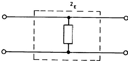
8. Add emitter feedback to device with shunt feedback,  $Z_{T2} = Z_E + Z_{T1}$ .
