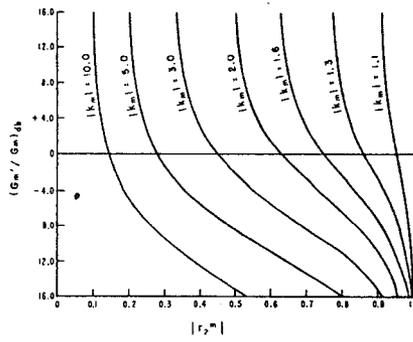
Fig. 6(b) — The curves shown for various values of  $|K_m| > 1$  can be used to obtain constant power gain circles on the  $r_2^m$  plane. This graph gives the radii of stable power gain for the case  $|K| > 1$  and  $K$  negative.
