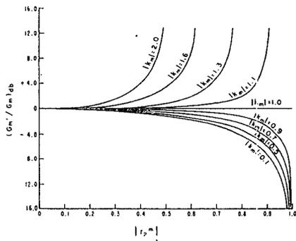
Fig. 6(a) — Set of curves giving the radii of constant power gain circles as a function of the load  $|r_2^m|$  with  $|k_m|$  as a parameter. This set of curves provides circles of positive power gain for  $K > 1$ .
