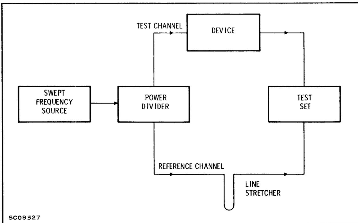
Figure 2. Setup for Measuring  $S_{12}$  and  $S_{21}$
