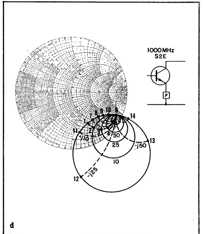
**Figs. 5a, b, c and d – Common emitter series feedback impedance mapped onto the s-parameter planes at 1 GHz. The shaded regions correspond to inductive impedance while the colored areas are capacitive.**
