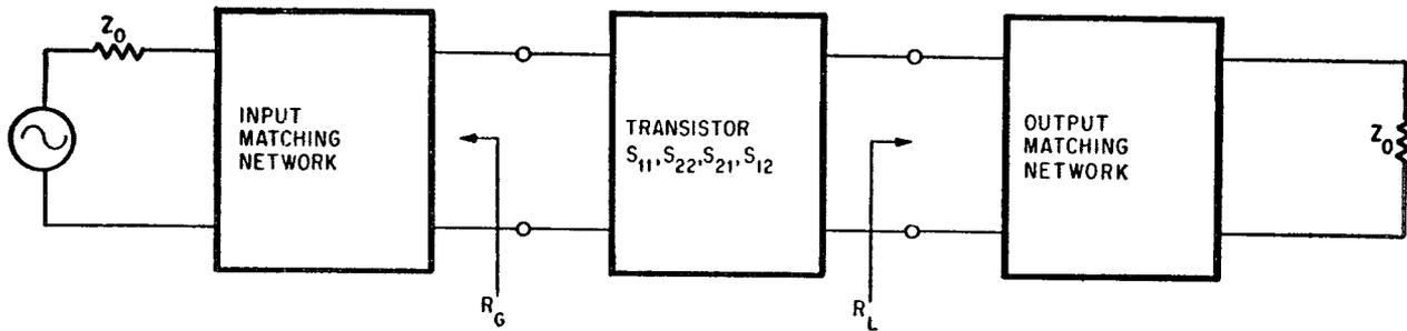
To design an amplifier stage, source and load impedances are found to give the gain desired. Then impedances are synthesized, usually as matching networks between a fixed impedance source or the load and the device. When using *s* parameters to design a transistor amplifier, it is advantageous to distinguish between a simplified or unilateral design for times when  $s_{12}$  can be neglected and when it must be used.
