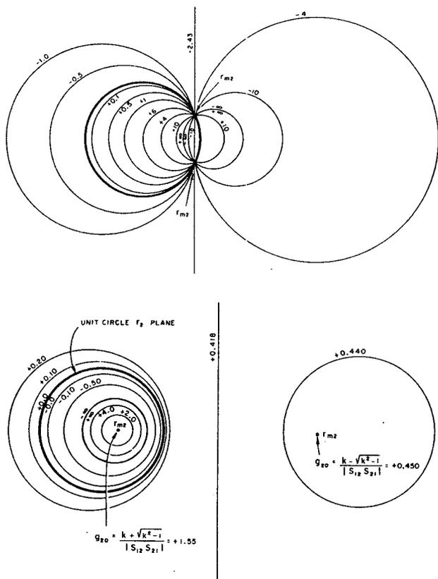
Fig. 10 — Constant gain circles ( $g_2$ ) for a set of  $s$  parameters which satisfy case C of Fig. 9. Gain  $g_2$  is given as a numerical ratio, not in dB. Circles are plotted on the  $r_2$  plane.  $s_{11} = 0.707 / 0^\circ$ ;  $s_{22} = 0.707 / 0^\circ$ ;  $s_{12} = 0.2 / 0^\circ$ .
