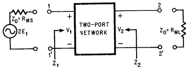
**Finding  $s_{21}$ .** By connecting a voltage source,  $2E_1$ , with the source impedance,  $Z_0$ , parameter  $s_{21}$  can be evaluated.
