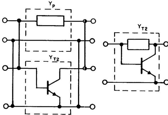
6. Convert  $Y$  matrix of device and shunt feedback to  $Z$  matrix,  $Y_{T2} \rightarrow Z_{T1}$ .
