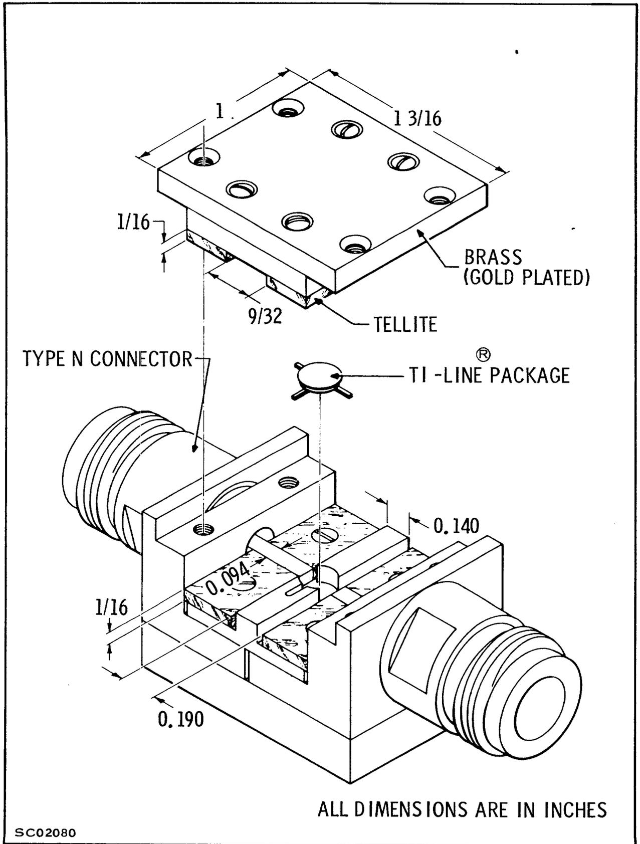
Figure 5. Improved TI-Line<sup>®</sup> Mount
