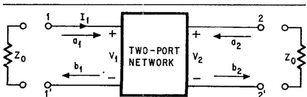
**Defining the s parameters.** Ratios of incident waves  $a_1$ ,  $a_2$  and reflected power waves  $b_1$ ,  $b_2$  for ports 1 and 2 define the four scattering parameters.
