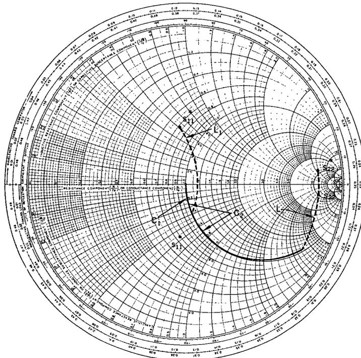
Fig. 6. Smith Chart for 300-MHz amplifier design example.
