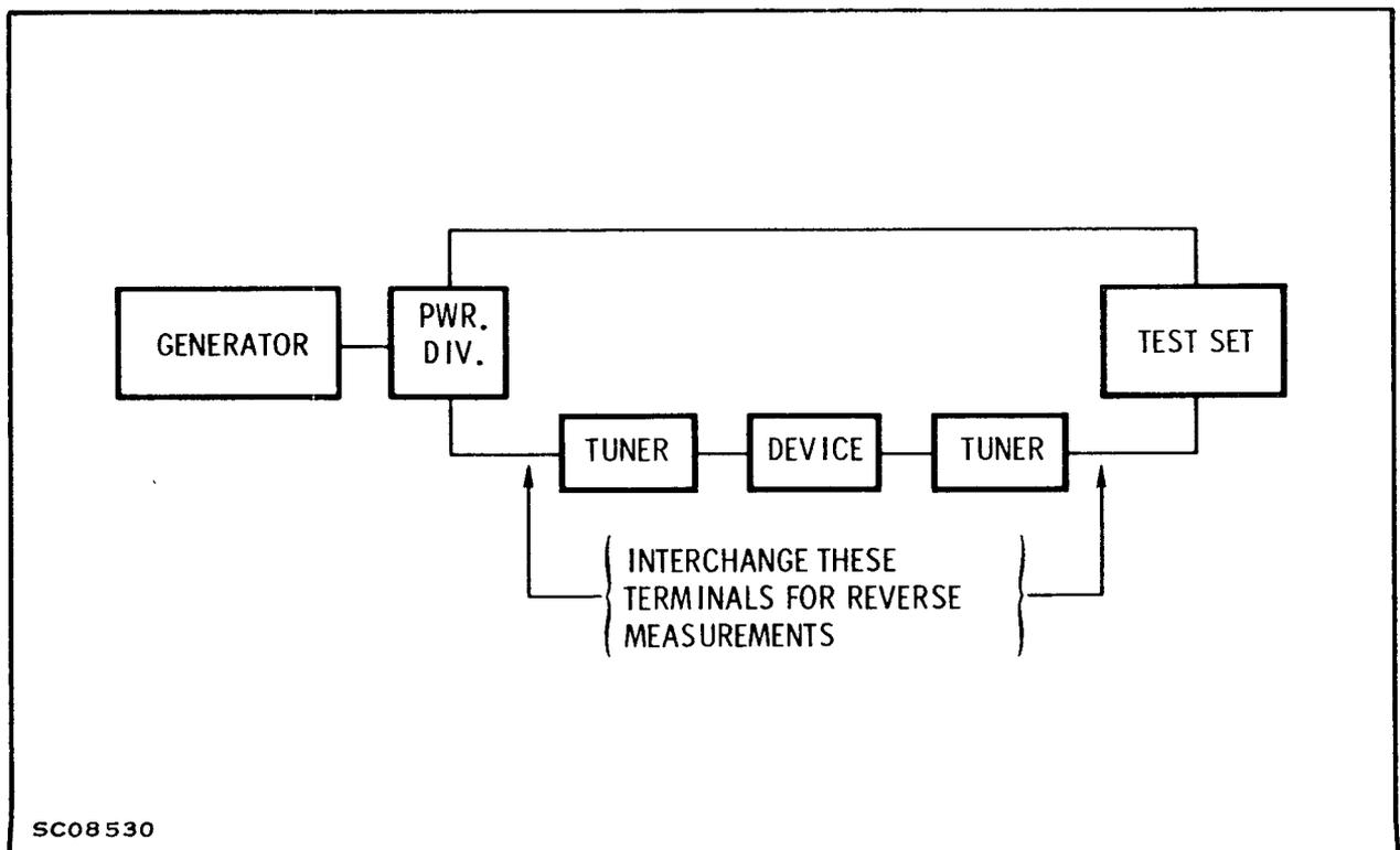
Figure 4. Setup for Measuring MSG, GMAX, K, U
