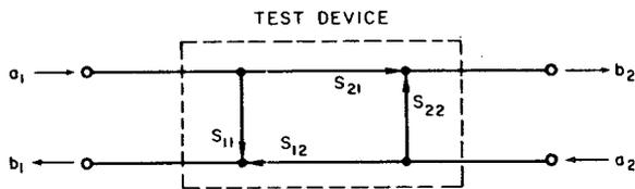
In this figure, a and b are the square roots of power;  $(a_1)^2$  is the power incident at port 1, and  $(b_2)^2$  is the power leaving port 2. The fraction of  $a_1$  that is reflected at port 1 is  $s_{11}$ , and the transmitted part is  $s_{21}$ . Similarly, the fraction of  $a_2$  that is reflected at port 2 is  $s_{22}$ , and  $s_{12}$  is transmitted in the reverse direction.
