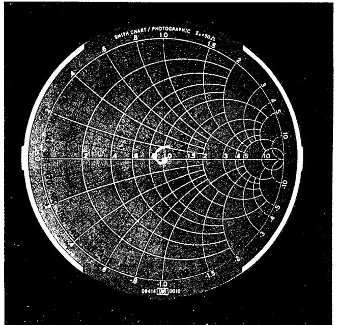
venience of polar display and swept measurement, you can get by with just the Vector Voltmeter (HP 8405, \$2750), top of the shelf to the left. It will work up to 1 GHz. A photo of a Smith chart overlay (white grid) of  $S_{22}$  over a 100 to 400 MHz range obtained by the author, Les Besser, is shown on the right.
