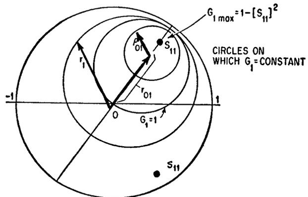
A graphical plot helps in design of an amplifier stage. Here the measured parameters  $s_{11}$  and  $s_{11}^*$  are plotted on a Smith chart. The upper point is  $s_{11}^*$ .
