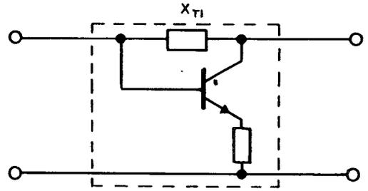
10. Set up  $X$  matrices for base and collector bias elements (may be complex),  $X_B$ ,  $X_C$ .
