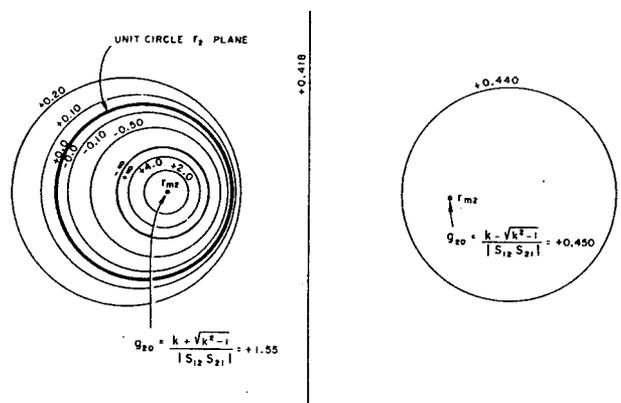
Fig. 11 — Constant gain circles for case B' of Fig. 9. The inside of the heavily lined circle provides positive real input impedance.  $s_{11} = -0.707$ ;  $s_{22} = 0.707$ ;  $s_{12} = 1.2$ ;  $r_{m2} = (3.53, 0.287)$ .
