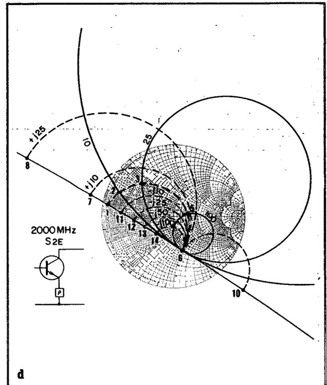
Figs. 8a, b, c and d - Common emitter shunt feedback impedance mapped onto the s-parameter planes at 2 GHz. The shaded regions correspond to inductive impedances while the colored areas are capacitive.
