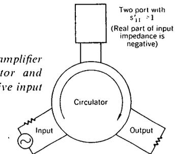
Fig. 11. Reflection amplifier consists of circulator and transistor with negative input resistance.
