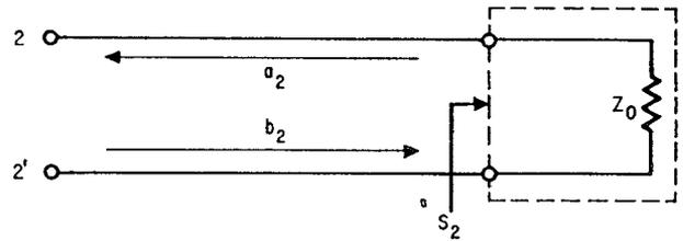
**Impedance matching.** By setting  $a_2$  equal to zero the engineer can determine the  $s_{11}$  value. The condition  $a_2 = 0$  implies that the reference impedance  $R_{MS}$  is set equal to the load impedance  $Z_0$ .
