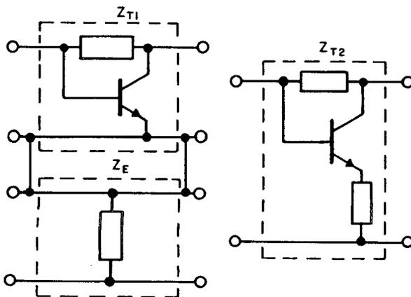
9. Convert  $Z$  matrix of device with feedbacks to  $X$  matrix,  $Z_{T2} \rightarrow X_{T1}$ .
