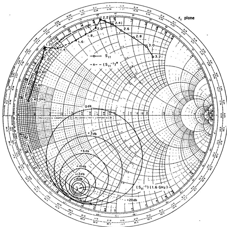
Fig. 5 — Plot of  $s_{11}$  vs. frequency for a transistor in common base showing frequency ranges over which the input is positive and negative real with  $50 \Omega$  on the output. Where the curve is dashed, the real part is read off as negative. Any generator placed on the device which lies outside the shaded region provides a total positive resistance at all frequencies. The circles indicate contours of constant gain at 1.6 GHz.
