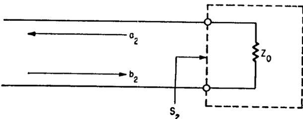
By setting  $a_2$  equal to zero the  $s_{11}$  parameter can be found. The  $Z_0$  resistor is thought of as a one-port network. The condition  $a_2 = 0$  implies that the reference impedance  $R_{02}$  is set equal to the load impedance  $Z_0$ . By connecting a voltage source,  $2 E_{01}$ , with the source impedance,  $Z_0$ , parameter  $s_{21}$  can be found using equation 5
