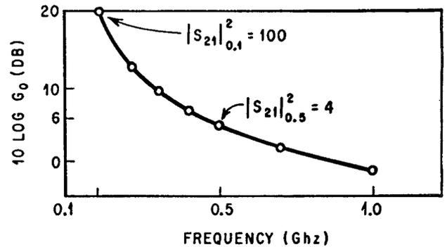
From the measured data transducer power gain is plotted as decibels versus frequency. From the plot an amplifier of constant gain is designed. Smith chart is used to plot the scattering parameters.
