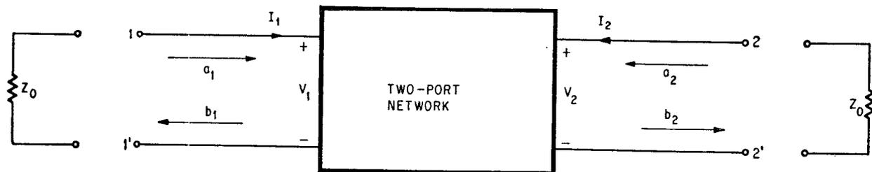
Scattering parameters are defined by this representation of a two-port network. Two sets of incident and reflected parameters  $(a_1, b_1)$  and  $(a_2, b_2)$  appear at terminals 1-1' and 2-2' respectively.
