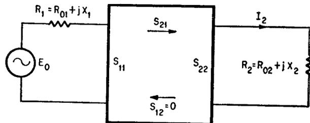
The two-port network is terminated at the ports by impedances containing resistance and reactance. Expressions for the transducer power gain can then be derived in terms of the scattering parameters.
