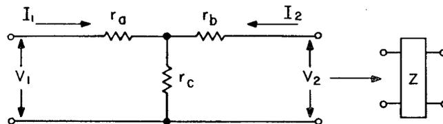
2. An equivalent  $Z$  matrix for a common resistive "T" is derived (in text) using the symbols defined above. All operations involve matrices; accordingly, the reader should familiarize himself with matrix algebra.
