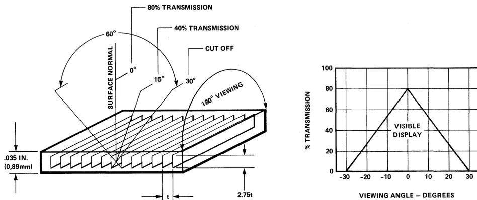
Figure 11. Construction characteristics of 0° neutral density louvered filter.
