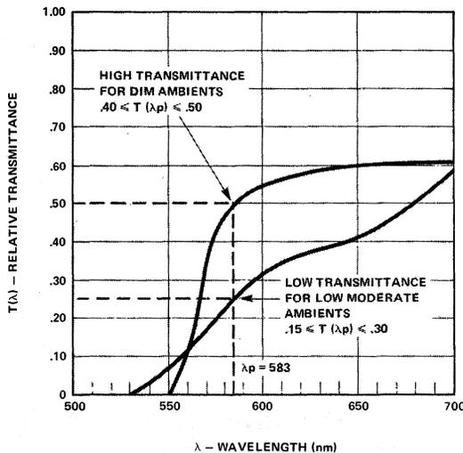
Figure 5. Typical transmittance curves for filters to be used with HP yellow displays.
