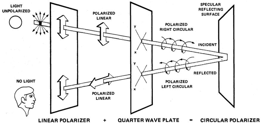
Figure 13. The operation of a circular polarizer.
