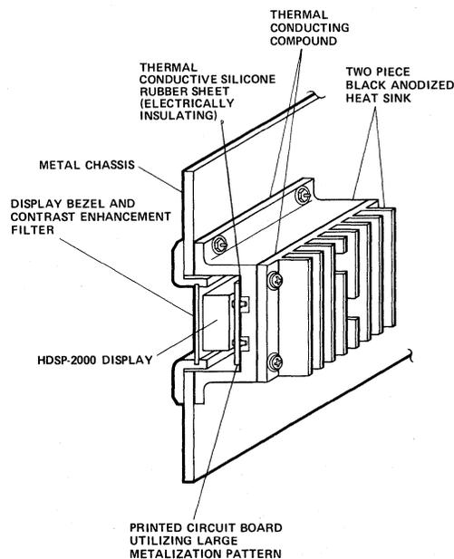
Figure 8. Two-Part Heat Sink for the HP HDSP-2000.
