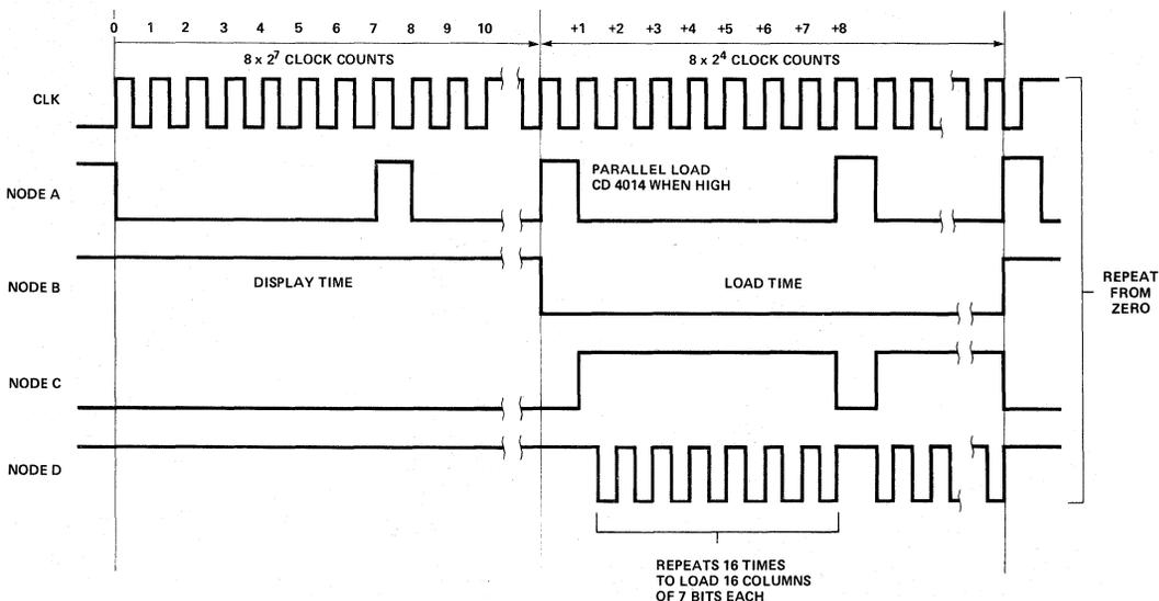
Figure 4. Timing Diagram for Display Interface.
