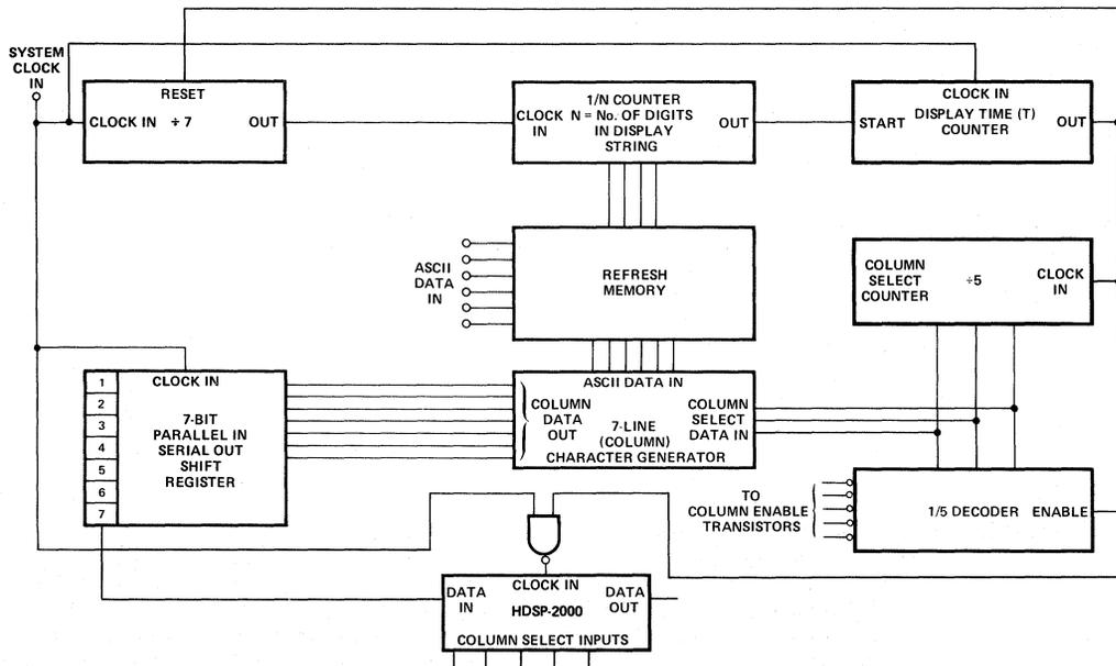
Figure 2. Block Diagram of a Basic Display System.
